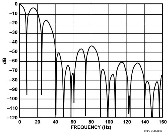
Figure 6. Frequency Response for a 16.6 Hz Update Rate
