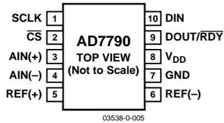
Figure 5. Pin Configuration
