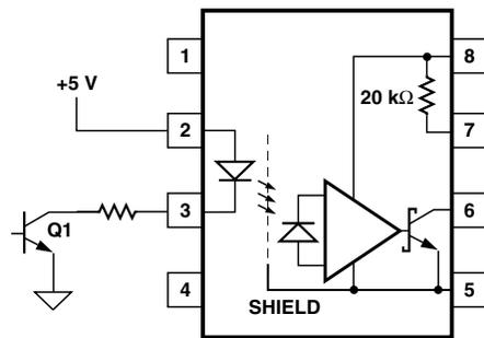
Figure 21. Not recommended open collector LED drive circuit.
