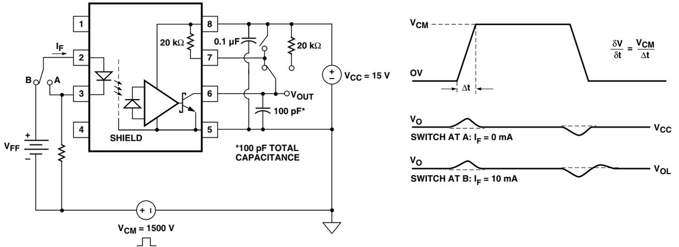
Figure 7. CMR test circuit. Typical CMR waveform.
