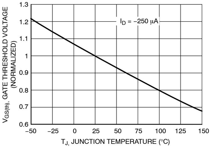
Figure 9. Gate Threshold Voltage Variation with Temperature
