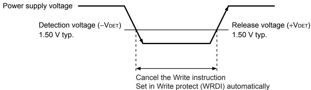
**Figure 19** Operation during Low Power Supply Voltage
