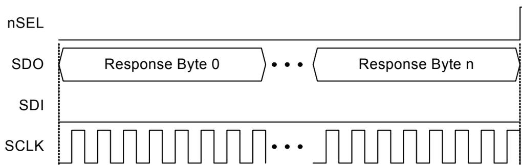
**Figure 10. SPI Read Command—Clock Out Read Data**
