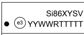
Figure 11.1. 8-Pin Narrow Body SOIC Top Marking
