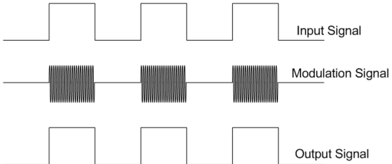
Figure 2.2. Modulation Scheme
