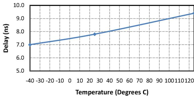
Figure 3.6. Propagation Delay vs. Temperature (5.0 V Data)
