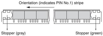
2) Tape and reel packing (surface-mount terminal type)
