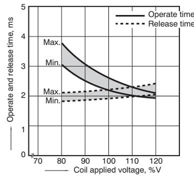
6-(2). Operate and release time (without diode)
