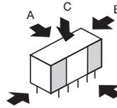
Please chuck the
