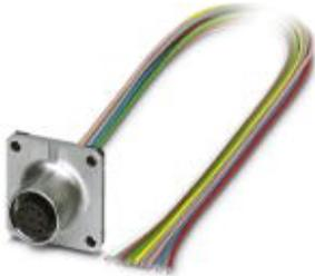
Sensor/actuator flush-type socket, 8-pos., M12, A-coded, front/square flange mounting, with 0.5 m TPE litz wire, 8 x 0.25 mm<sup>2</sup>
