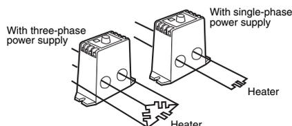
Pass the lines through the openings only once. If they are passed more than once, the actual operating current will be less than the set current. The lines can be passed in either direction.
