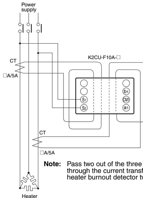
**Note:** Pass two out of the three line conductors through the current transformers of the heater burnout detector twice as shown.
