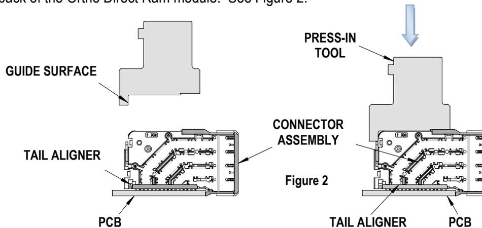
3. Using the application tool and an appropriate press, seat the Ortho Direct Ram module until there is less than 0.10mm (.004) in clearance between the bottom of the aligner and the surface of the PCB. See Figure 3.
