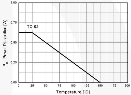
Figure 10. Power Dissipation vs. Ambient Temperature
