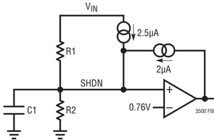
Figure 8. Undervoltage Lockout
