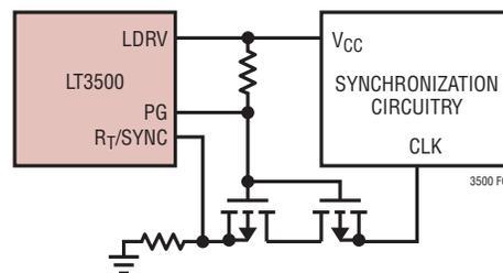
Figure 7. Synchronous Signal Powered from Regulator's Output
