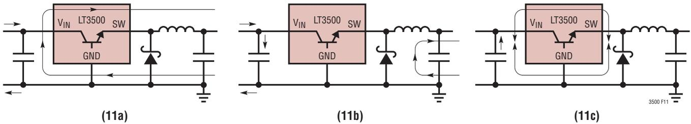
**Figure 11. Subtracting the Current when the Switch is On (11a) from the Current when the Switch is Off (11b) Reveals the Path of the High Frequency Switching Current (11c). Keep this Loop Small. The Voltage on the SW and BST Traces will Also be Switched; Keep These Traces as Short as Possible. Finally, Make Sure the Circuit is Shielded with a Local Ground Plane**
