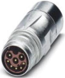
Coupler connector, straight, SPEEDCON locking, M17, Number of positions: 17, Type of contact: Male connector, Crimp connection, shielded: yes, Cable diameter: 3.5 mm...5.5 mm
