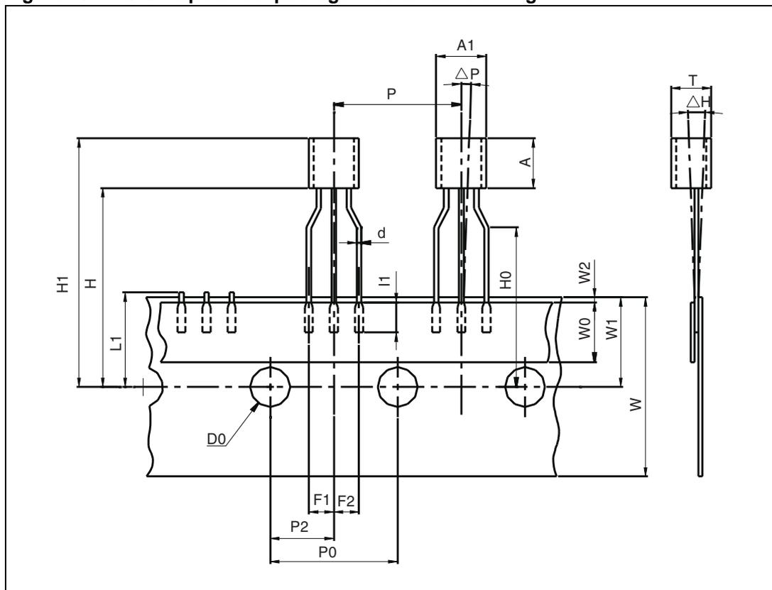
Table 4. TO-92 tape &amp; reel package mechanical data
