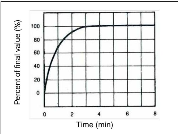
Figure 11. Thermal response in stirred oil bath
