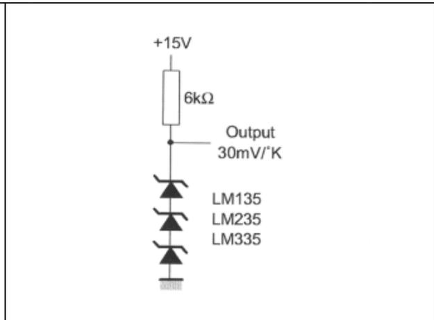
Figure 17. Isolated temperature sensor
