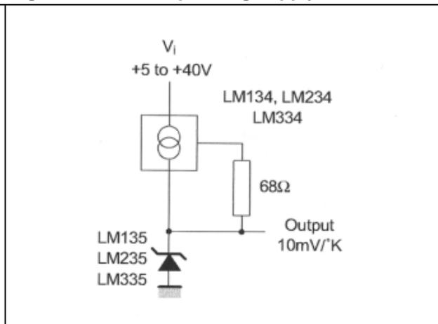
Figure 15. Calibrated sensor
