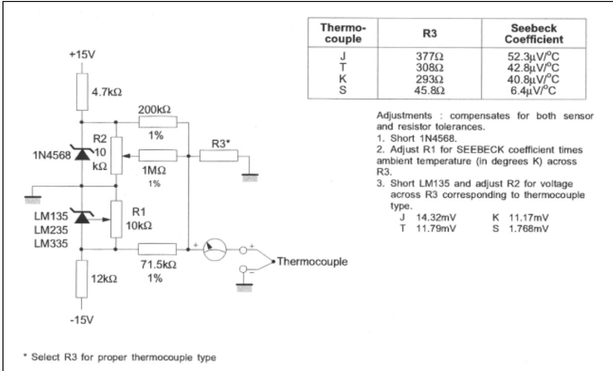
Figure 22. Single power supply cold junction compensation
