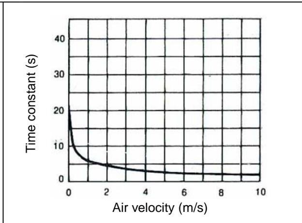
Figure 10. Thermal response in still air
