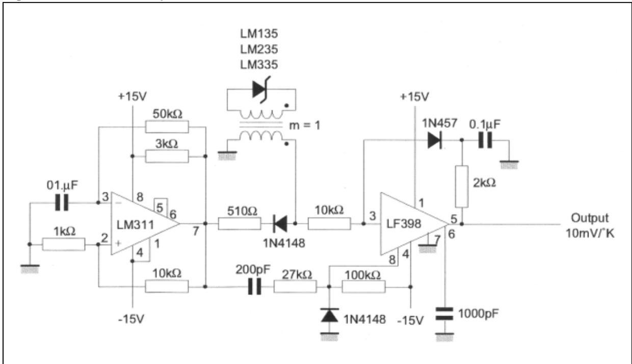
Figure 18. Simple temperature controller
