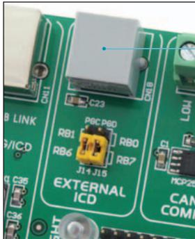
Figure 4-1: Pins RB6 and RB7 are used for programming
