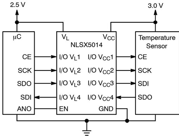
Figure 3. Application Example for  $V_L < V_{CC}$
