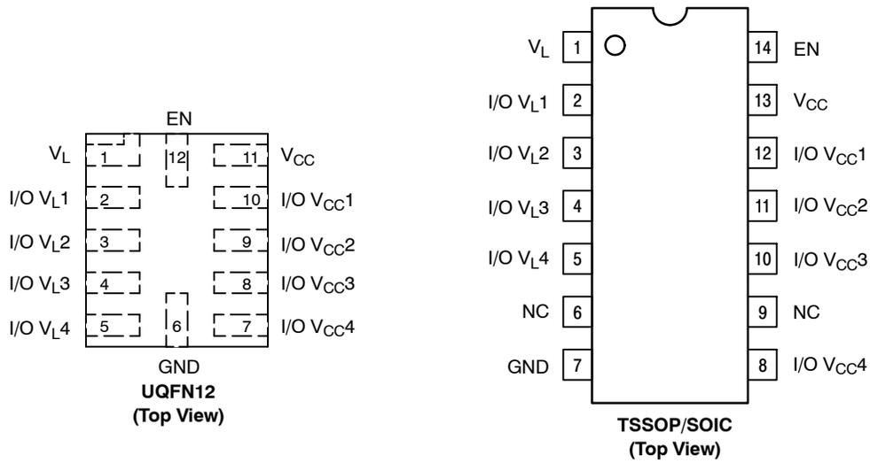
Figure 1. Pin Assignments
