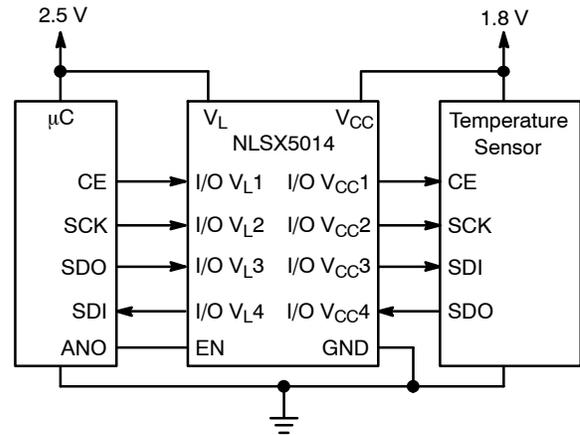
Figure 4. Application Example for  $V_L > V_{CC}$
