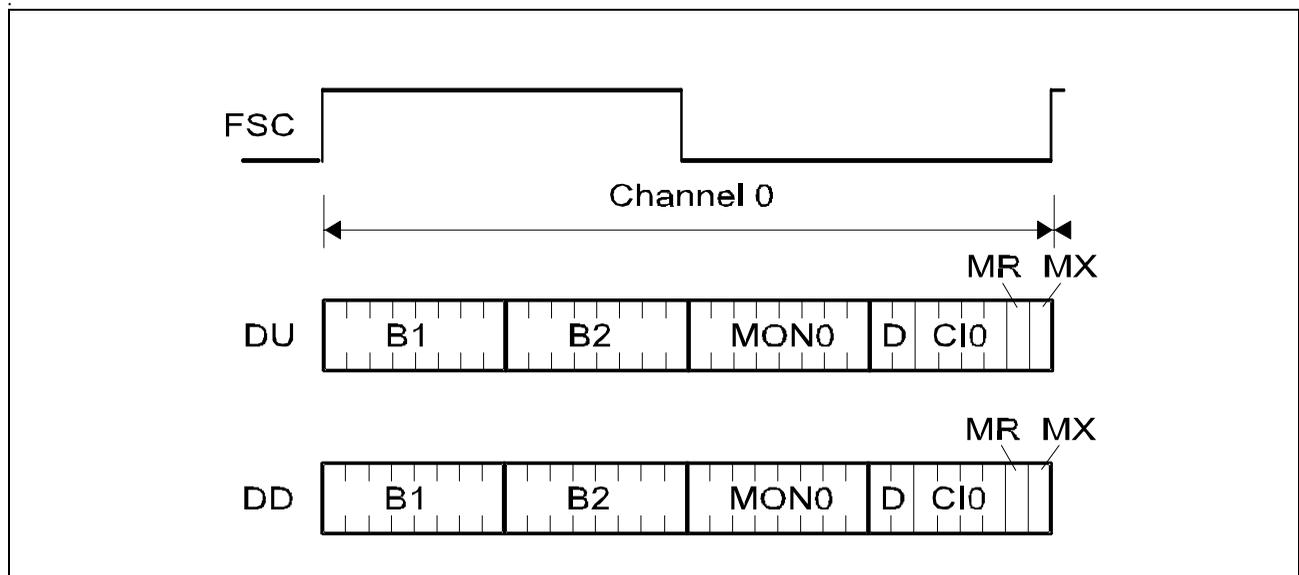
**Figure 4 IOM<sup>®</sup>-2 Frame Structure of the Q-SMINT<sup>®</sup>O**
