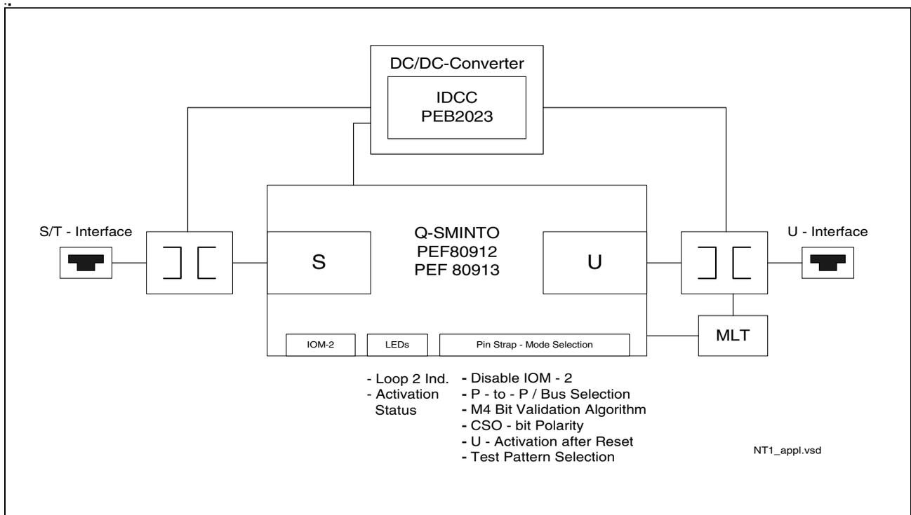
Figure 3 Application Example Q-SMINT<sup>®</sup>O: Standard NT1
