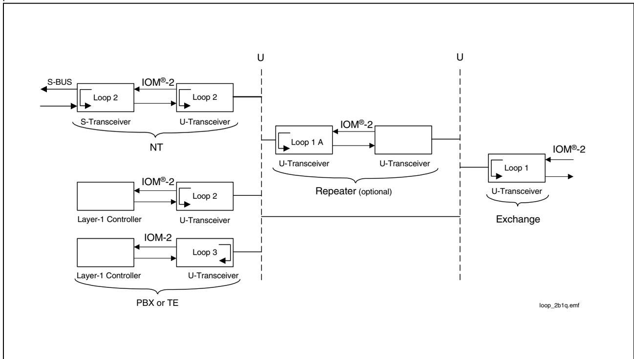
**Figure 24 Test Loopbacks**
