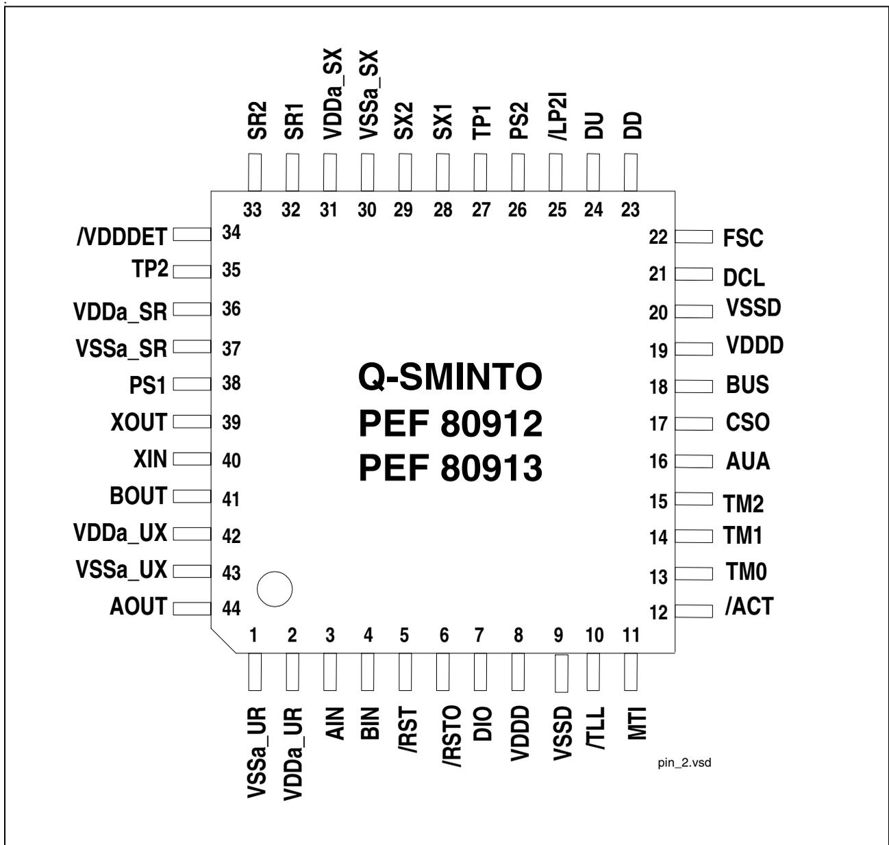
Figure 1 Pin Configuration
