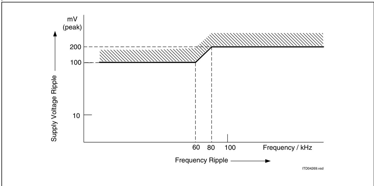
Figure 30 Maximum Sinusoidal Ripple on Supply Voltage
