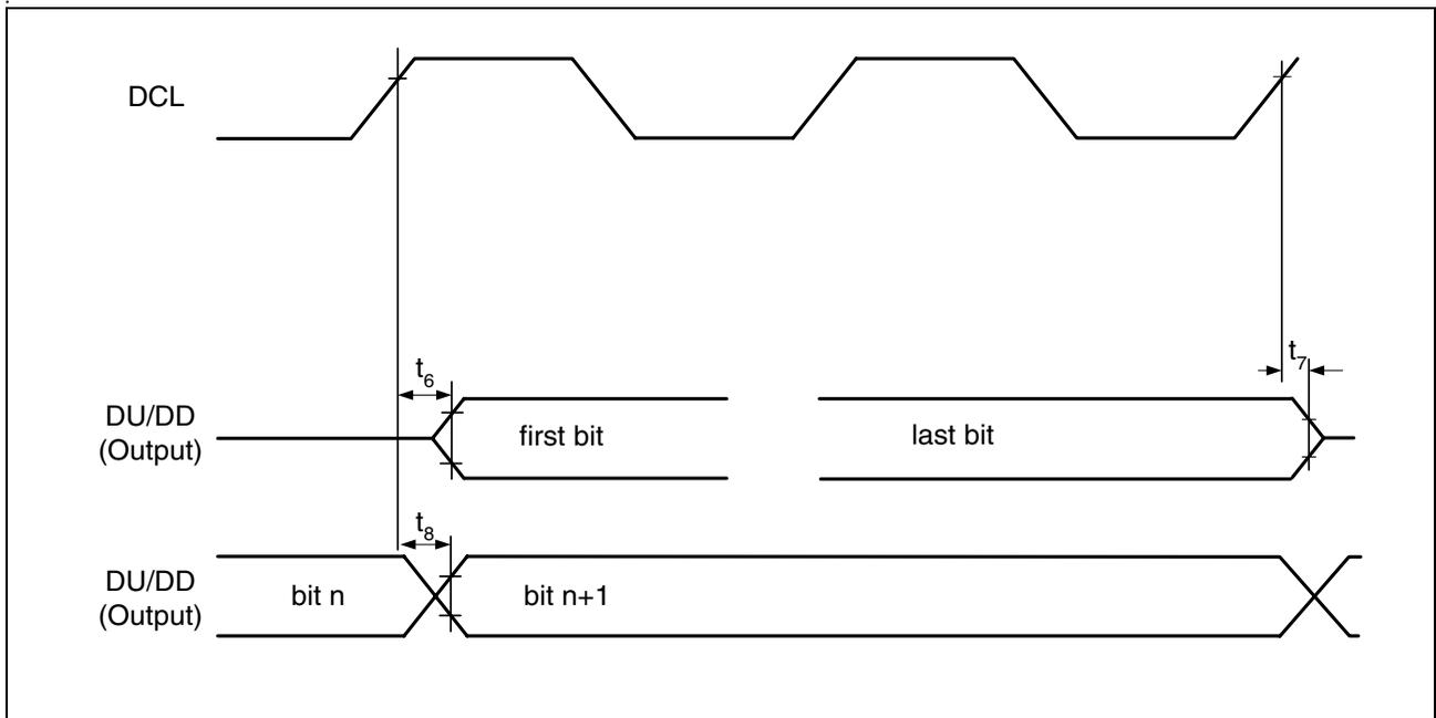
**Figure 32 IOM<sup>®</sup>-2 Interface - Bit Synchronization Timing**
