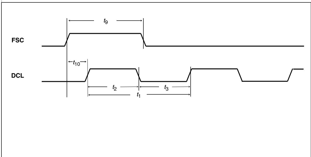
**Figure 33 IOM-2 Interface - Frame Synchronization Timing**
