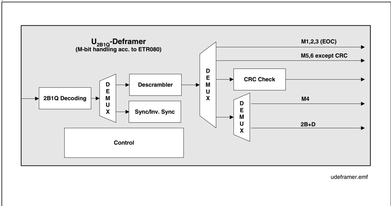
Figure 8 U<sub>2B1Q</sub> Deframer - Data Flow Scheme
