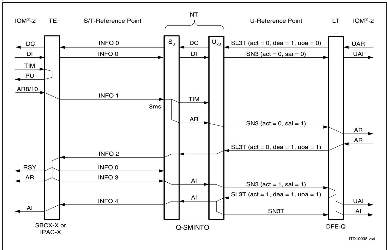
Figure 21 Activation from TE with U Active
