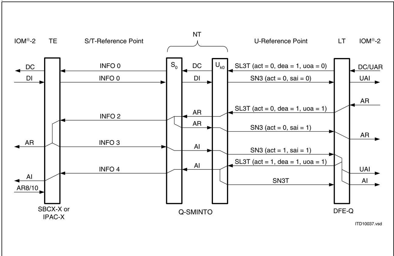
Figure 20 Activation from LT with U Active
