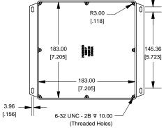
Black Textured Polyester Powder Paint - RAL 9011 1590FFBK Unfinished 1590WFF 1590WFFBK **Black Textured Powder Paint** Recommended Torque: 75 ozf.in / 55 cN.m Black Textured Cover Screws (Pkg 50) 1590WMS100BK [6-32 x 1/2" SS Type 304] Unfinshed Cover Screws (Pkg 100) 1590WMS100 [6-32 x 1/2" Nickel Plated Screws] Standard Cover Screws
