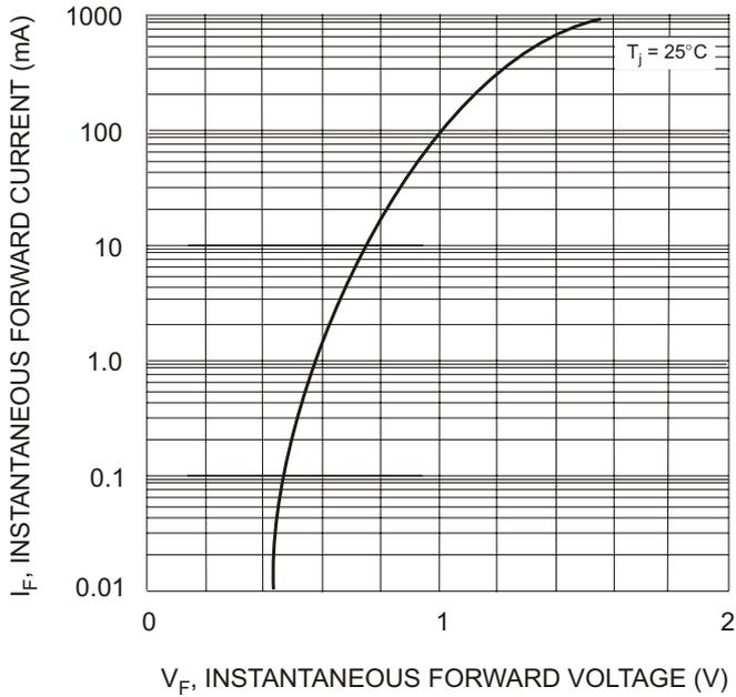
Fig. 1 Forward Characteristics
