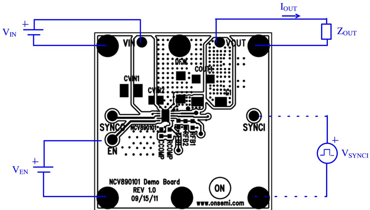
Figure 3. NCV890101GEVB Board Connections
