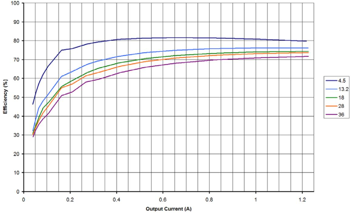
Figure 4. Efficiency at 2 MHz for a 3.3 V output
