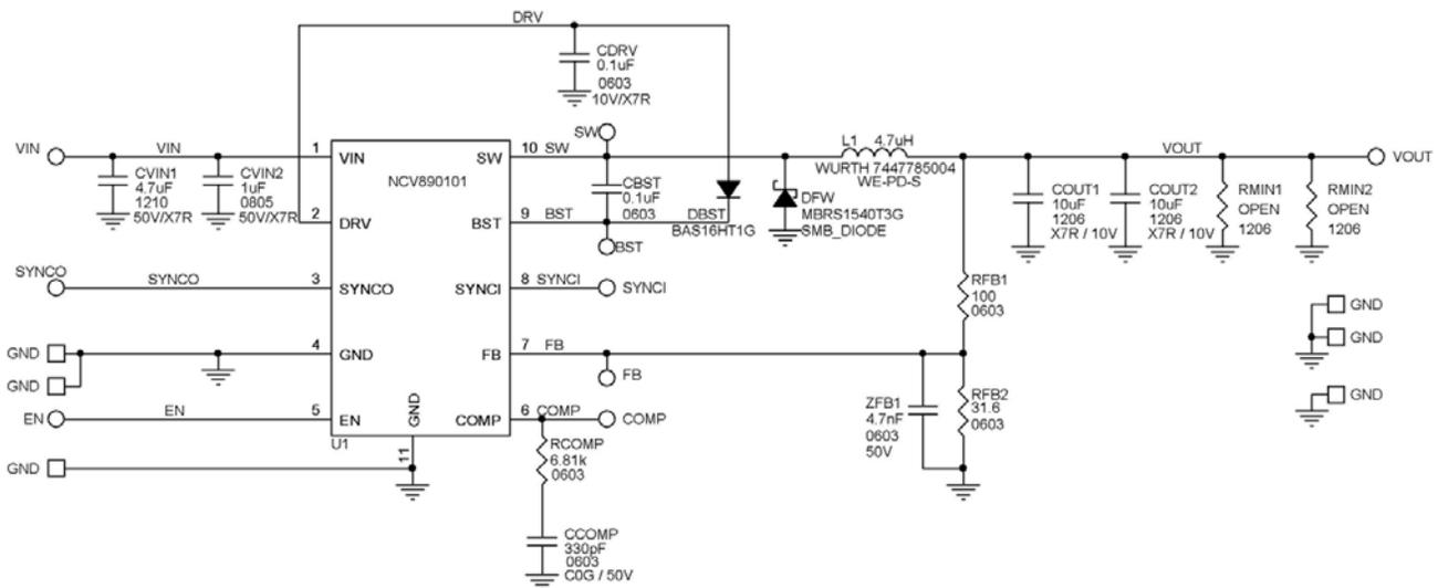
Figure 2. NCV890101GEVB Board Schematic
