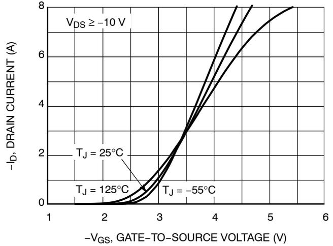
Figure 2. Transfer Characteristics
