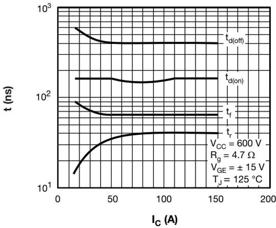
Fig. 7 - Typical Switching Time vs.  $I_C$
