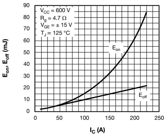
Fig. 3 - Switching Loss vs. Collector Current
