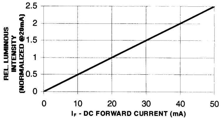
Fig 2. Rel. Luminous Intensity vs. DC Forward Current
