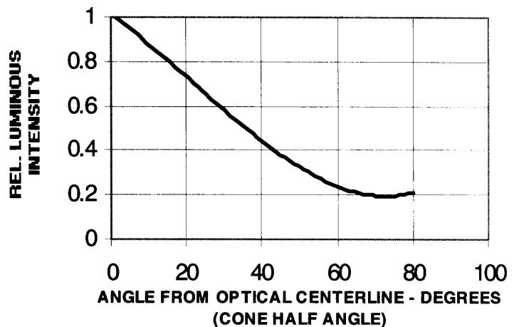
Fig 4. Rel. Luminous Intensity vs. Angular Displacement
