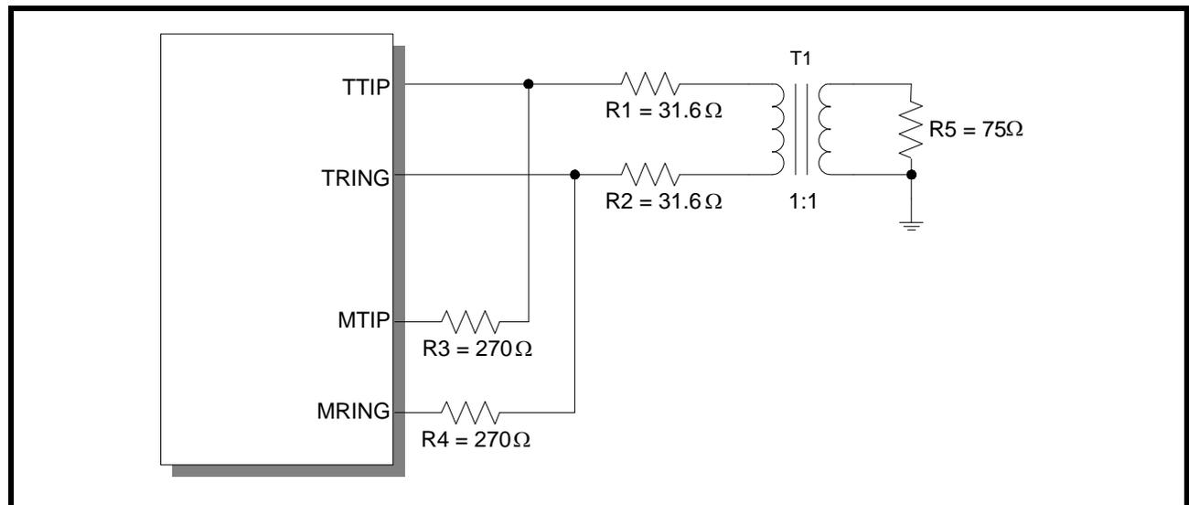
When the Transmit Drive Monitor circuitry is connected to the line as illustrated in Figure 26, then it monitors the line for transitions. As long as the Transmit Drive Monitor circuitry detects transitions on the line via the MTIP and MRING pins, it keeps the DMO (Drive Monitor Output) signal “Low”. However, if the Transmit Drive Monitor circuit detects no transitions on the line for 128±32 TCLK periods, then the DMO signal toggles “High”.
