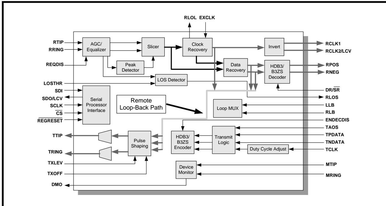
During Remote Loop-Back operation, any data which is inputted via the RTIP and RRING input pins is also outputted to the Terminal Equipment via the RPOS, RNEG and RCLK output pins.
