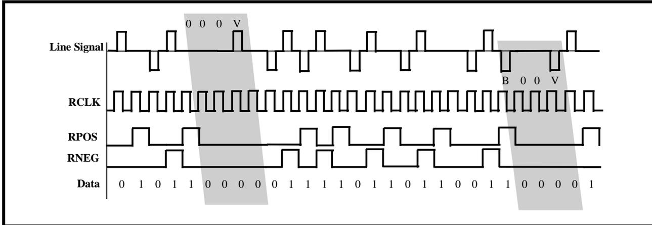
**NOTE:** If the HDB3 Decoder detects any bipolar violation (e.g., “V”) pulses that is not in accordance with the HDB3 Line Code format, or if the HDB3 Decoder detects a string of 4 (or more) “0’s” in the incoming line signal, then the HDB3 Decoder flags this event as a Line Code Violation by pulsing the LCV output pin “High”.
