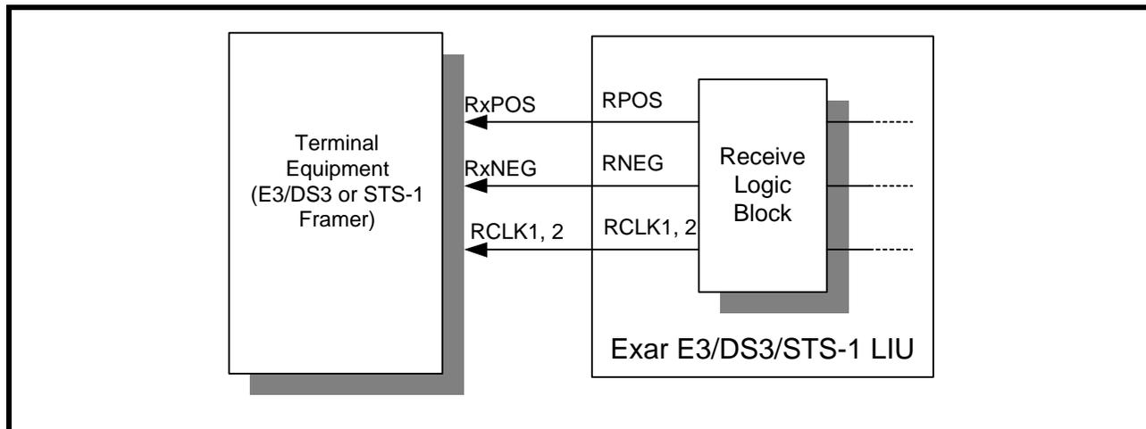
The manner that the LIU transmits Dual-Rail data to the Receiving Terminal Equipment is described below and illustrated in Figure 25. The XRT73LC00A typically updates the data on the RPOS and RNEG output pins on the rising edge of RCLK1 (or RCLK2).
