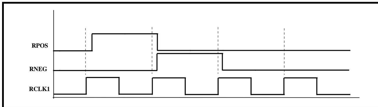
RCLK1 (or RCLK2) is the Recovered Clock signal from the incoming Received line signal. These clock signals are typically 34.368 MHz for E3 applications, 44.736 MHz for DS3 applications and 51.84 MHz for SONET STS-1 applications.
