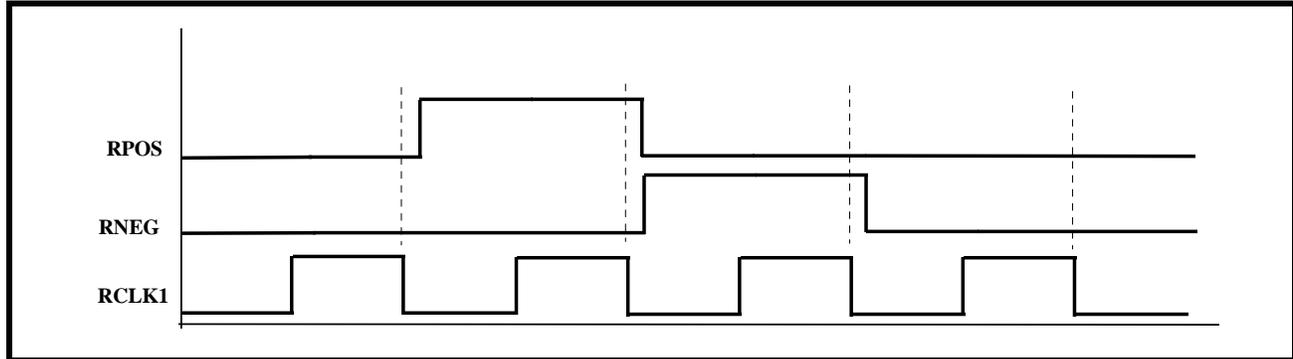
To configure the XRT73LC00A to invert the RCLK1 output signal, the XRT73LC00A must be operating in the HOST Mode. This configuration can be implemented by accessing the Microprocessor Serial Interface block and writing a “1” into the RCLK1INV bit-field in Command Register CR3 to invert RCLK1.
