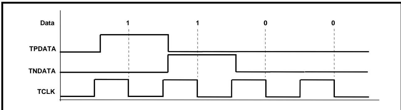
The manner that the LIU handles Dual-Rail data is described below and illustrated in Figure 12. The XRT73LC00A typically samples the data on the TPDATA and TNDA input pins on the falling edge of TCLK.
