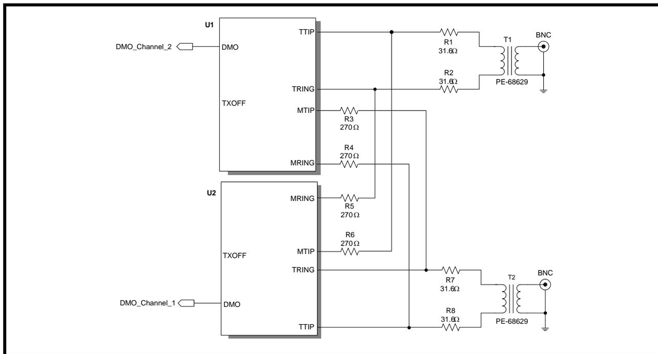
Presented in Figure 33, if LIU # 1 (U1) fails, then LIU # 2 (U2) drives its DMO output pin “High”. Likewise, if LIU # 2 (U2) fails, then LIU # 1 (U1) drives its DMO output pin “High”.
