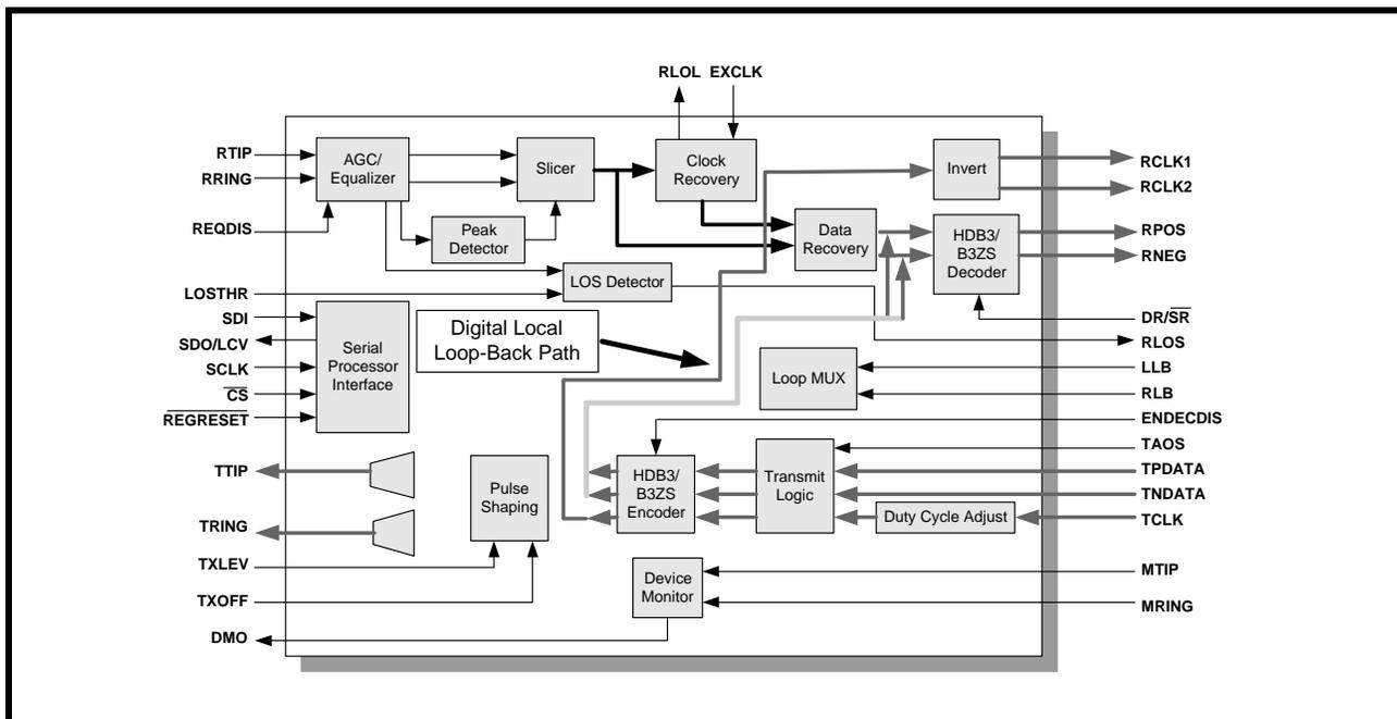
The Digital Local Loop-Back Mode, along with the TxOFF feature, is useful in Redundancy System Design. These two features permit the system to execute some diagnostic tests in the Back-up Line Card without transmitting data onto the line and interfering with the DS3/E3/STS-1 traffic from the Primary Line Card.
