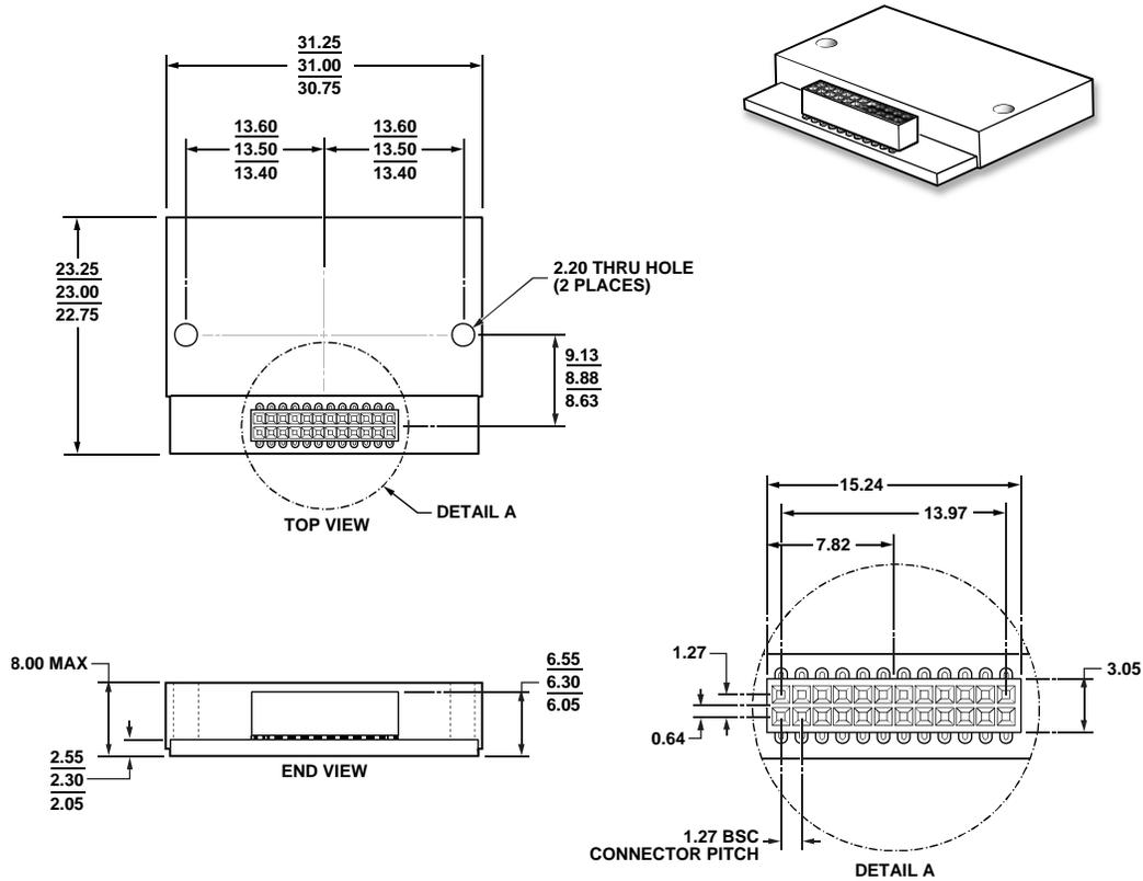
Figure 21. 24-Lead Module with Connector Interface (ML-24-4)
