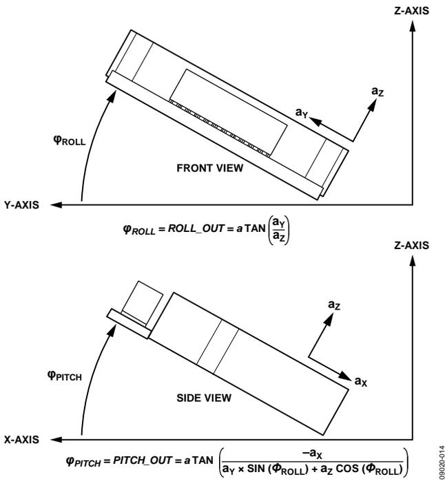
Figure 14. Orientation for PITCH\_OUT and ROLL\_OUT Angles
