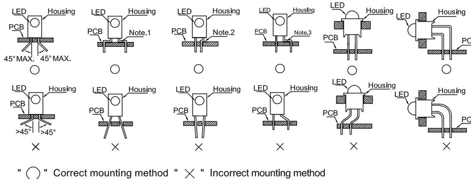
Note 1-3: Do not route PCB trace in the contact area between the leadframe and the PCB to prevent short-circuits.
