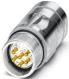
Coupling connector, straight, shielded: yes, SPEEDCON locking, M23, Number of positions: 8+1, Type of contact: Male connector, Solder connection, Cable diameter: 10 mm ... 14.5 mm
