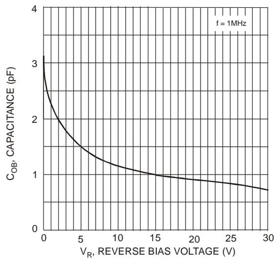
Fig. 4 Output Capacitance
