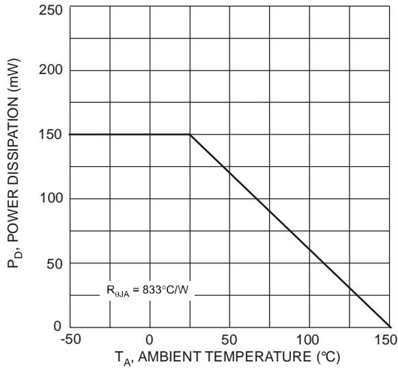
Fig. 1 Derating Curve
