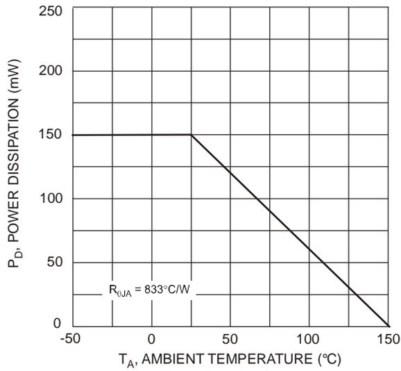
Fig. 1 Derating Curve
