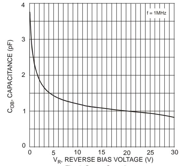
Fig. 4 Output Capacitance
