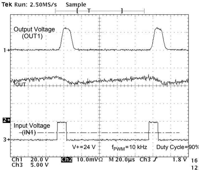
Figure 15. Output Voltage and Current vs. Input Voltage at V<sub>+</sub> = 24 V, PMW Frequency of 10 kHz, and Duty Cycle of 90%
