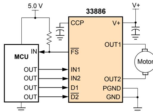
Figure 1. 33886 Simplified Application Diagram
