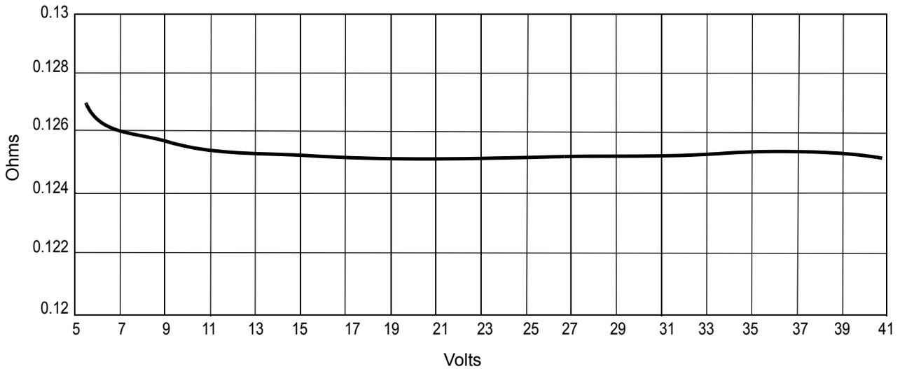
**Figure 19. Typical Low Side  $R_{DS(ON)}$  Versus  $V+$**
