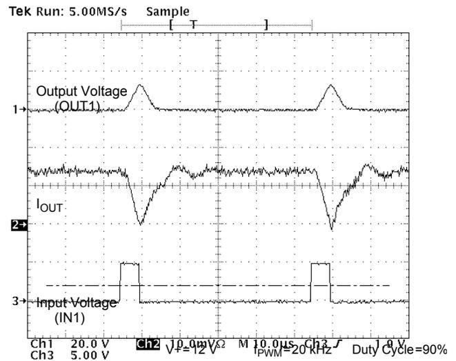
Figure 17. Output Voltage and Current vs. Input Voltage at V<sub>+</sub> = 12 V, PMW Frequency of 20 kHz, and Duty Cycle of 90% for a Purely Resistive Load
