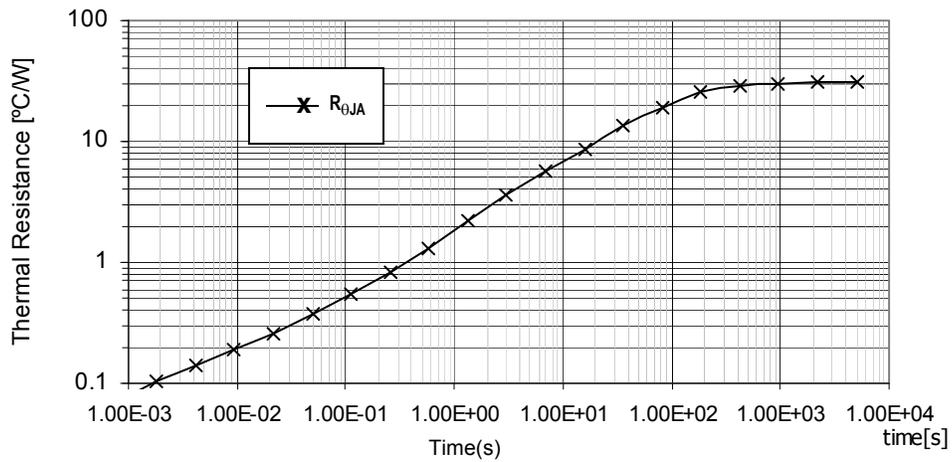
Figure 27. Transient Thermal Resistance  $R_{\theta JA}$
