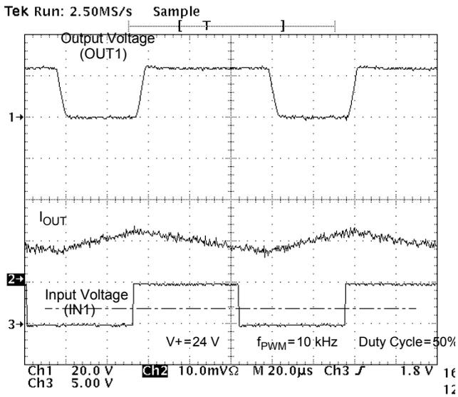
Figure 14. Output Voltage and Current vs. Input Voltage at V<sub>+</sub> = 24 V, PMW Frequency of 10 kHz, and Duty Cycle of 50%
