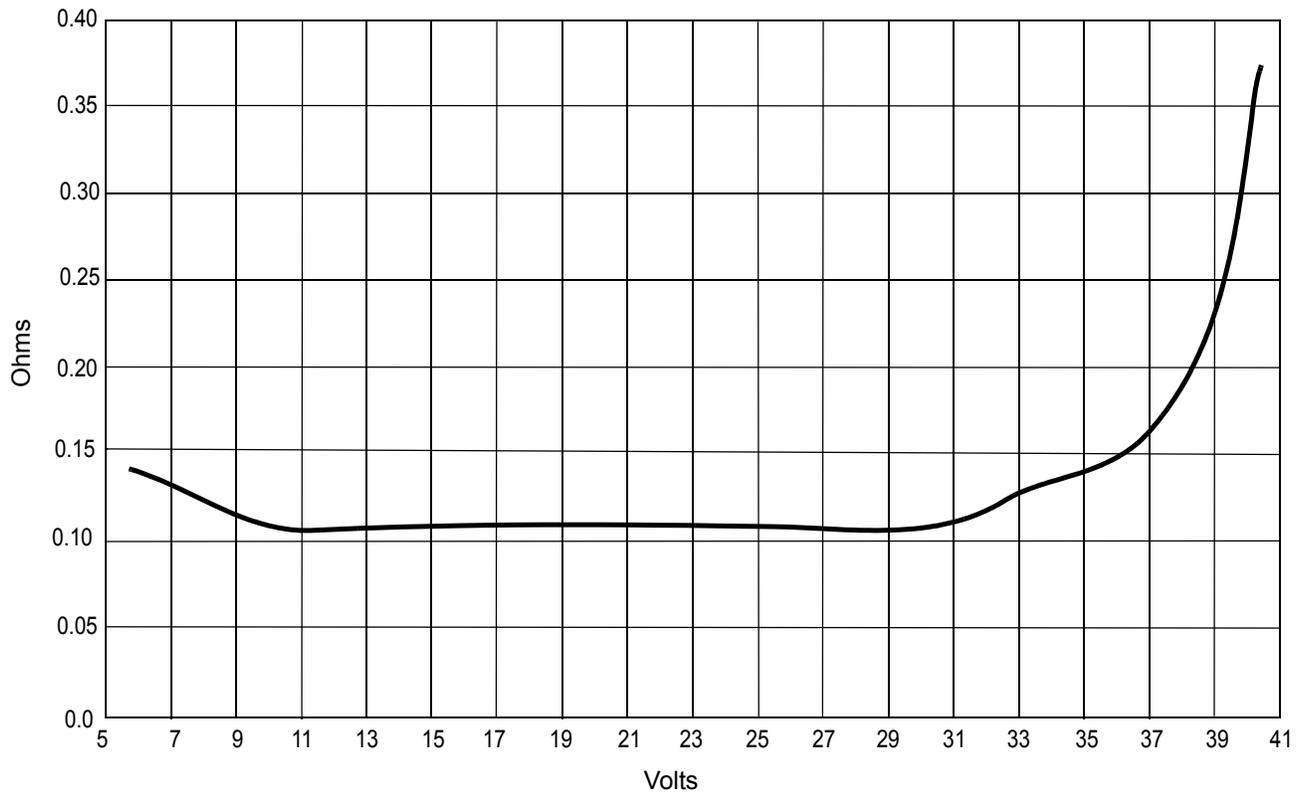
**Figure 18. Typical High Side  $R_{DS(ON)}$  Versus  $V+$**
