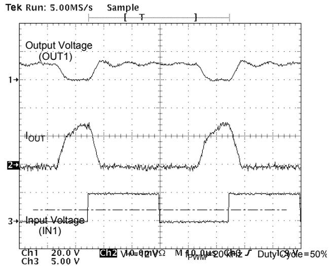
Figure 16. Output Voltage and Current vs. Input Voltage at V<sub>+</sub> = 12 V, PMW Frequency of 20 kHz, and Duty Cycle of 50% for a Purely Resistive Load
