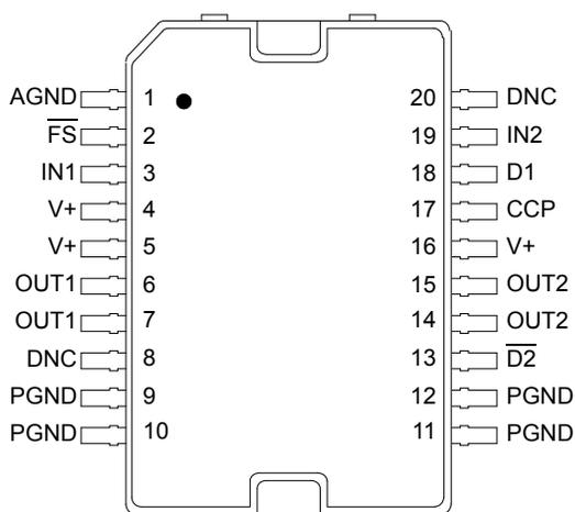
Figure 3. 33886 Pin Connections
