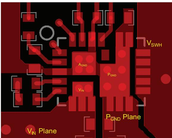
1. Thermal relief vias can be added on the  $V_{IN}$  and  $A_{GND}$  pads to utilize inner layers for high-current and thermal dissipation.
