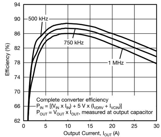
**Fig. 11 - Efficiency vs. Output Current ( $V_{IN} = 19\text{ V}$ )**
