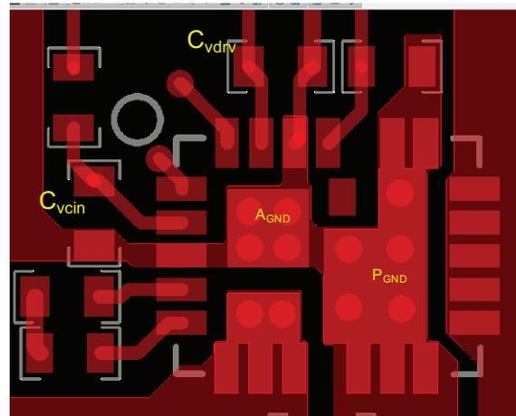
1. The  $V_{CIN}$  /  $V_{DRV}$  input filter ceramic cap should be placed as close as possible to the IC. It is recommended to connect two capacitors separately.
