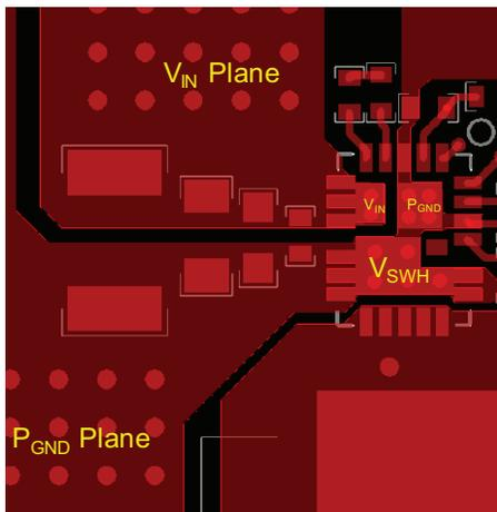
1. Layout  $V_{IN}$  and  $P_{GND}$  planes as shown above.
