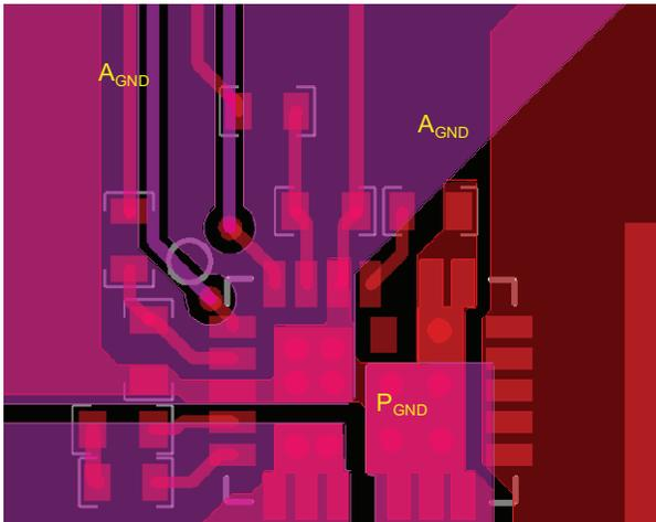
1. Route the PWM and ZCD\_EN# signal traces out of the top left corner next to pin 1.
