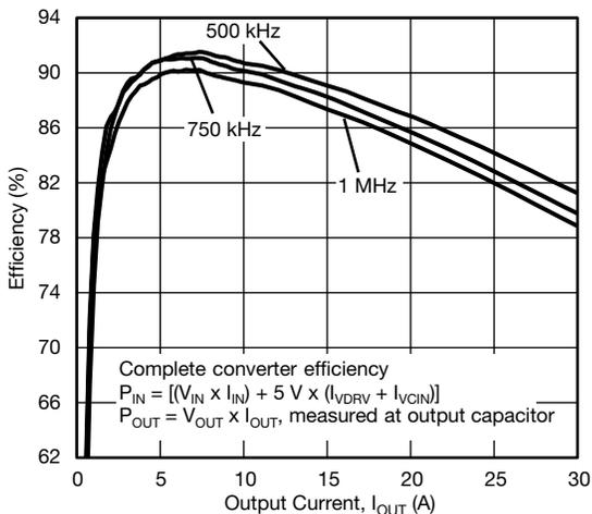
**Fig. 8 - Efficiency vs. Output Current ( $V_{IN} = 9\text{ V}$ )**
