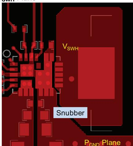
1. Connect output inductor to IC with large plane to lower resistance.
