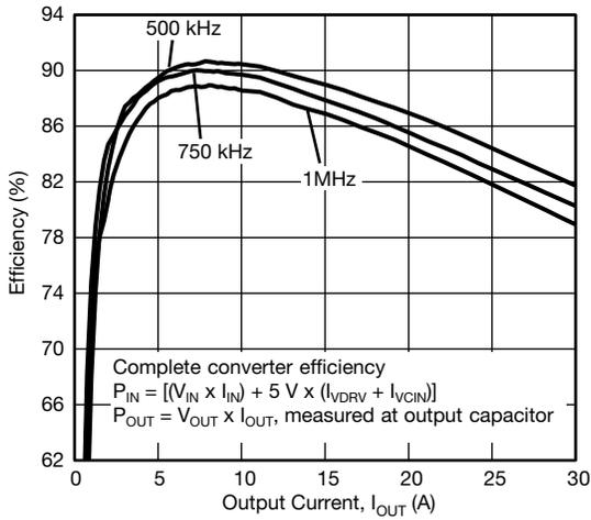
**Fig. 6 - Efficiency vs. Output Current ( $V_{IN} = 12.6\text{ V}$ )**
