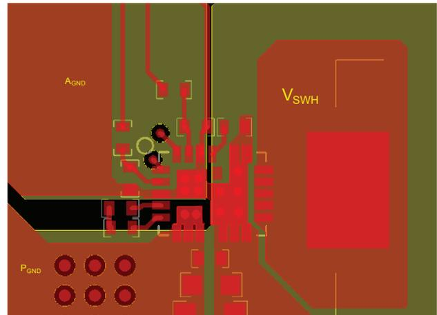
1. It is recommended to make a single connection between  $A_{GND}$  and  $P_{GND}$  which can be made on the top layer.
