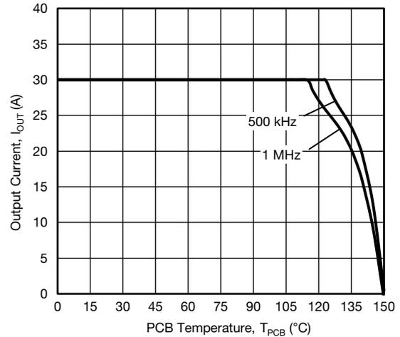
**Fig. 9 - Safe Operating Area ( $V_{IN} = 12.6\text{ V}$ )**
