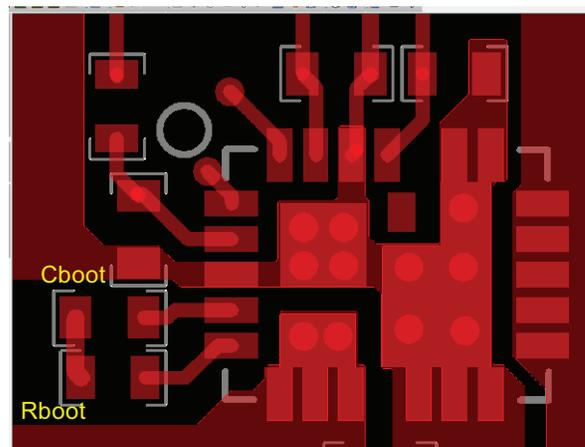
1. The components need to be placed as close as possible to IC, directly between PHASE (pin 5) and BOOT (pin 4).
