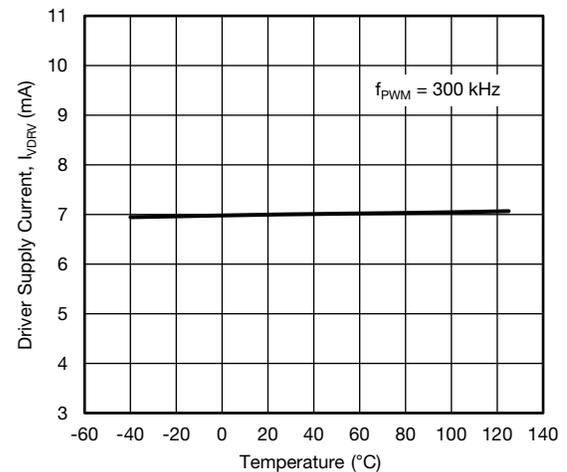
**Fig. 16 - Driver Supply Current vs. Temperature**
