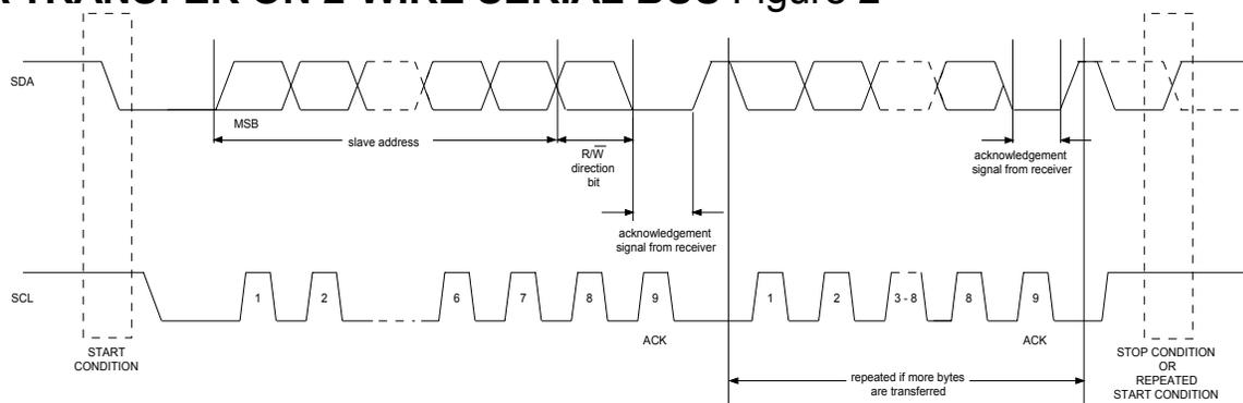
Figure 2 details how data transfer is accomplished on the 2-wire bus. Depending upon the state of the  $\overline{R/W}$  bit, two types of data transfer are possible:
