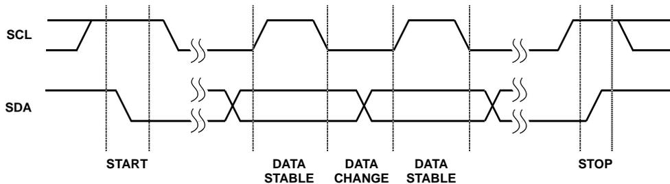
FIGURE 12. VALID DATA CHANGES, START AND STOP CONDITIONS
