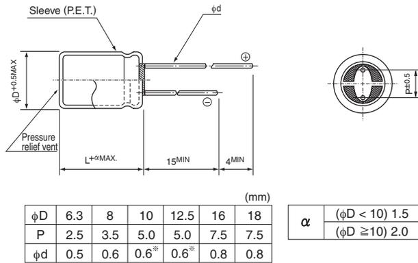
\* In case L>25 for the φ10 and φ12.5 dia unit, lead dia φd=0.8
