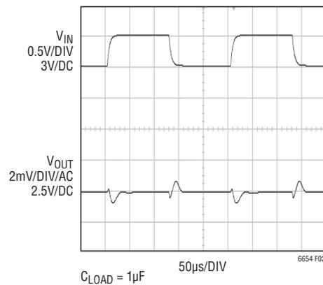
Figure 2. Output Response to  $0.5\text{V}$  Ripple on  $V_{\text{IN}}$
