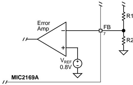
**Figure 2. Voltage-Divider Configuration**
