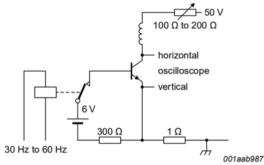
Fig. 4. Test circuit for collector-emitter sustaining voltage
