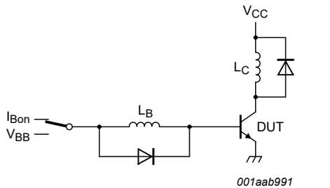
$V_{CC} = 300\text{ V}; V_{BB} = -5\text{ V}; L_C = 200\text{ }\mu\text{H}; L_B = 1\text{ }\mu\text{H}$
