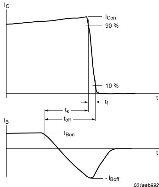
Fig. 11. Switching times waveforms for inductive load
