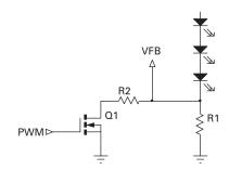
$$\begin{array}{cc} \text{MOSFET 'off'} \\ I_{LED(MIN)} & \frac{V_{FB}}{R_{LED}} \\ \text{MOSFET 'on'} \\ I_{LED(MAX)} & \frac{V_{^{FB}}}{R_{LED}} & I_{LED(MIN)} \end{array}$$
