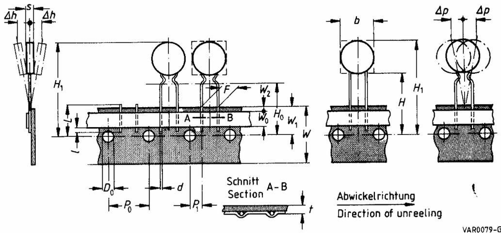
**Tape dimensions, in Millimeters (mm)**
