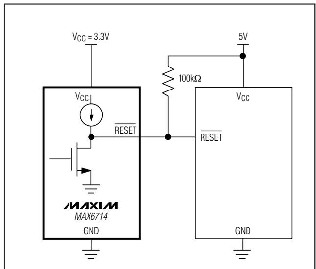
Figure 9. Interfacing to Different Logic Supply Voltage
