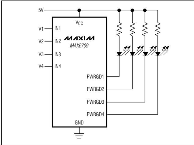
Figure 3. Quad Undervoltage Detector with LED Indicators
