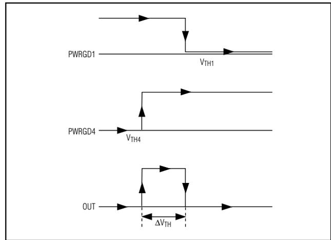
Figure 6. Output Response of Window Detector Circuit
