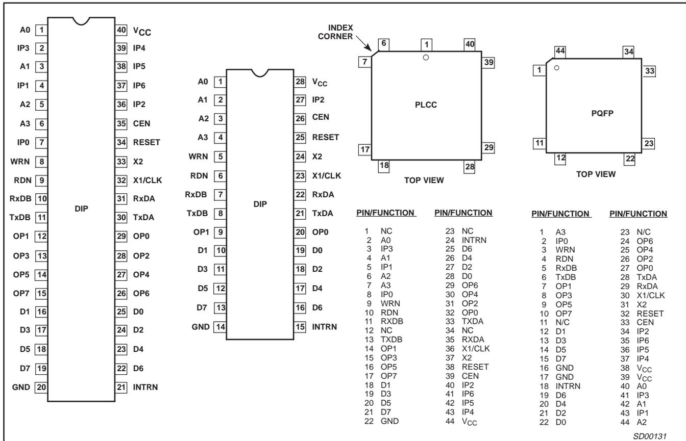
Figure 1. Pin Configurations
