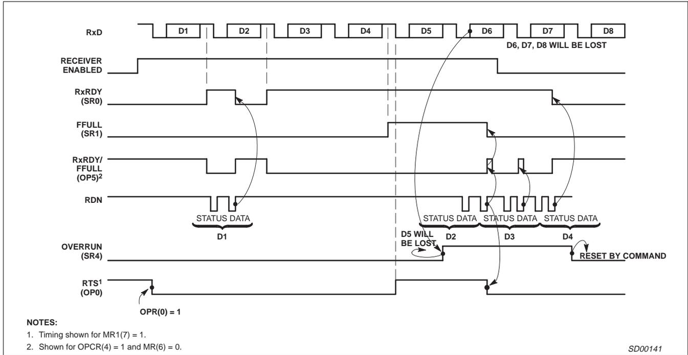
Figure 11. Receiver Timing
