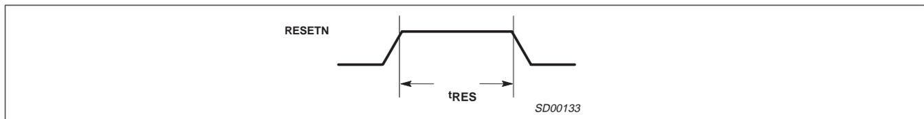
Figure 3. Reset Timing
