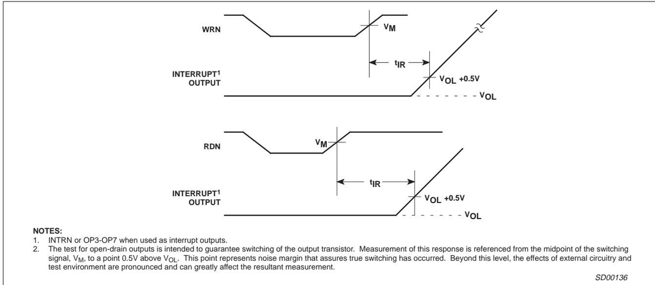
Figure 6. Interrupt Timing
