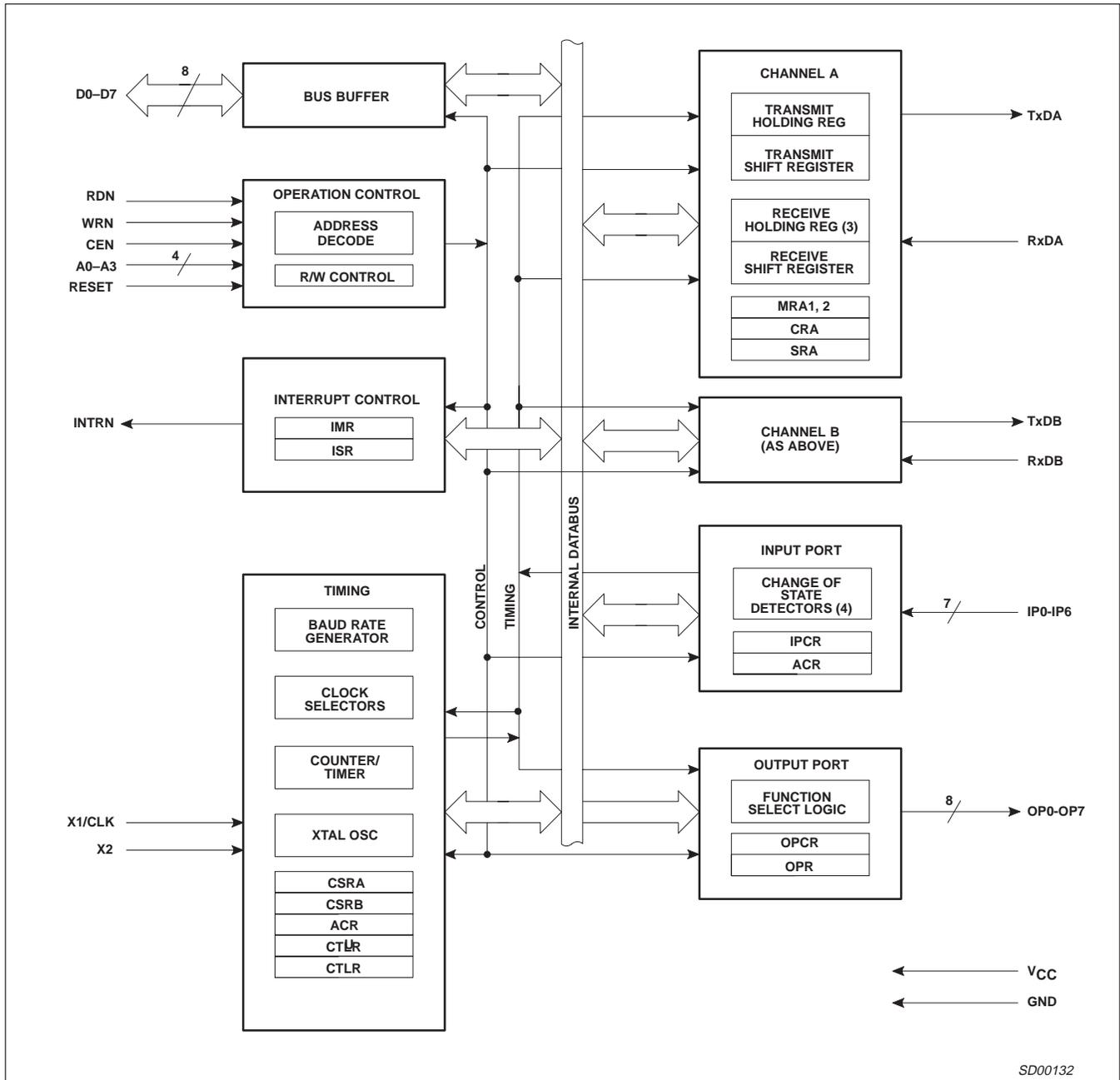
Figure 2. Block Diagram
