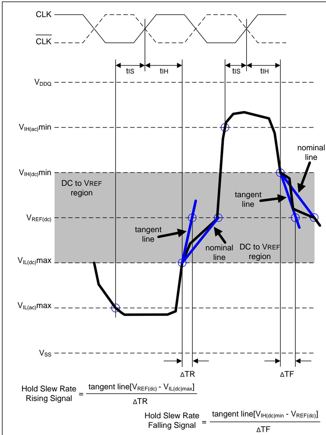
Figure 23 – Illustration of tangent line for t<sub>IH</sub>
