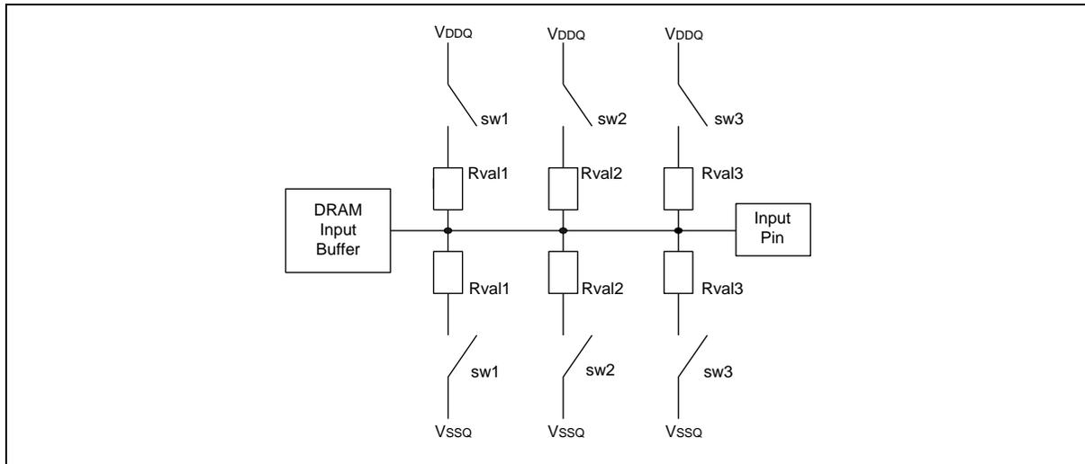
Switch (sw1, sw2, sw3) is enabled by ODT pin.
