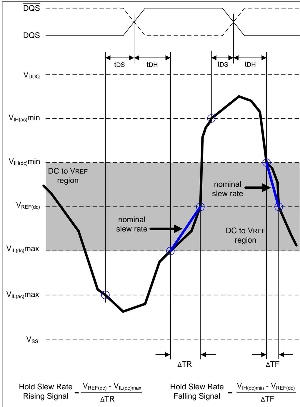
Figure 26 – Illustration of nominal slew rate for t<sub>DH</sub> (differential DQS,  $\overline{DQS}$ )
