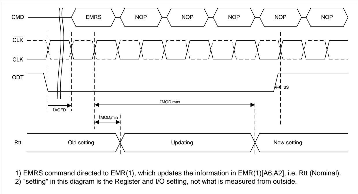
**Figure 10 – ODT update delay timing - tMOD**
