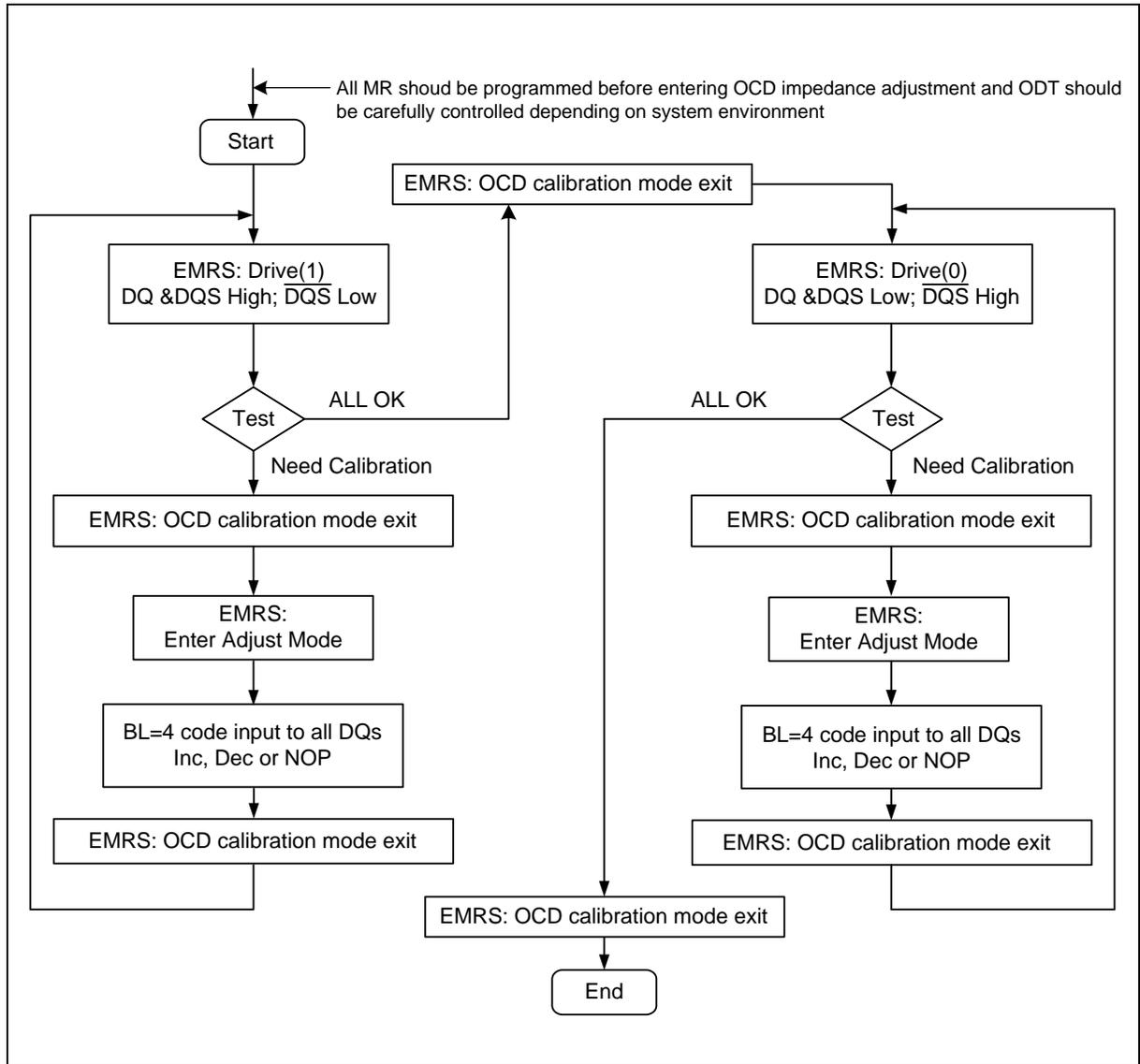
**Figure 6 – OCD Impedance Adjustment Flow Chart**
