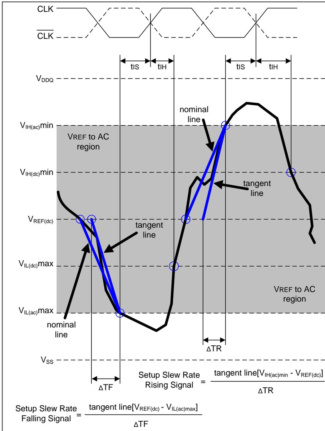
Figure 21 – Illustration of tangent line for t<sub>IS</sub>
