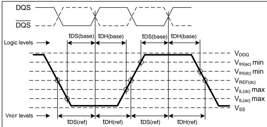
**Figure 19 – Differential input waveform timing – tDS and tDH**
