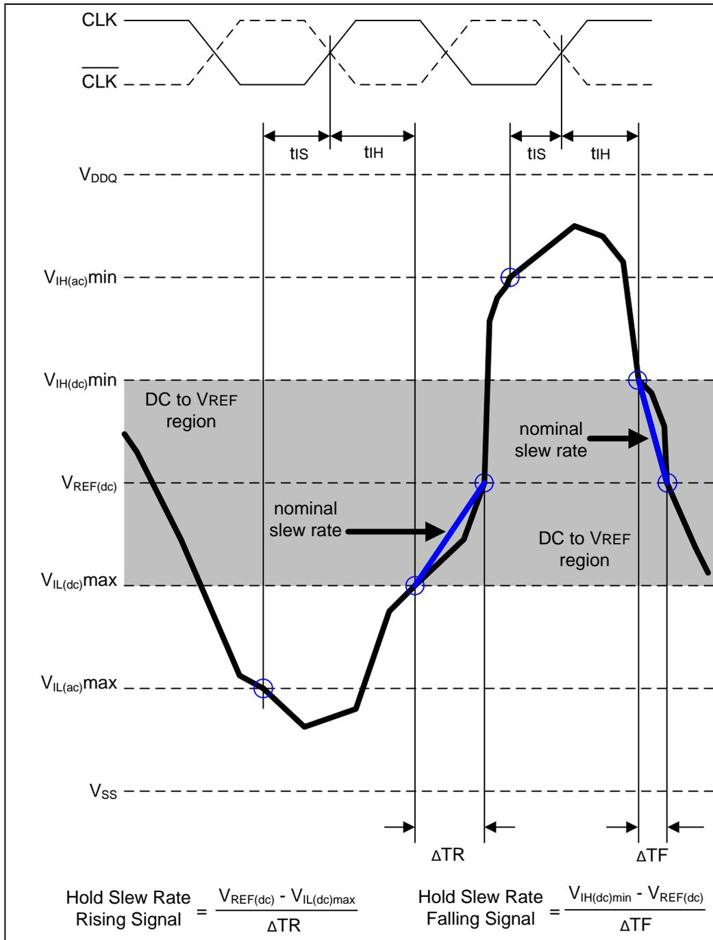
Figure 22 – Illustration of nominal slew rate for t<sub>IH</sub>
