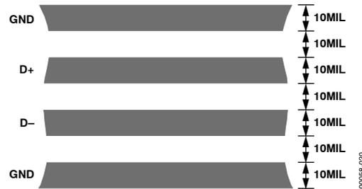
Figure 20. Arrangement of Signal Tracks
