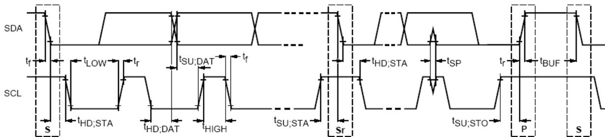
Figure 6. Definition of Timing for Full-Speed Mode Devices on the I<sup>2</sup>C Bus<sup>®</sup>
