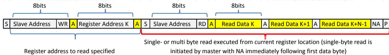
**Note:** If register is not specified, master begins reading from current register. In this case, only red bracketed sequence is needed.
