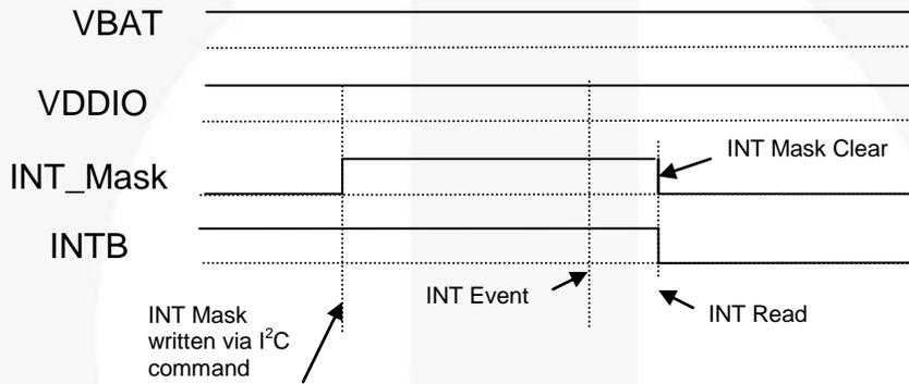
Figure 8. INT Mask to INTB Interrupt Timing Diagram
