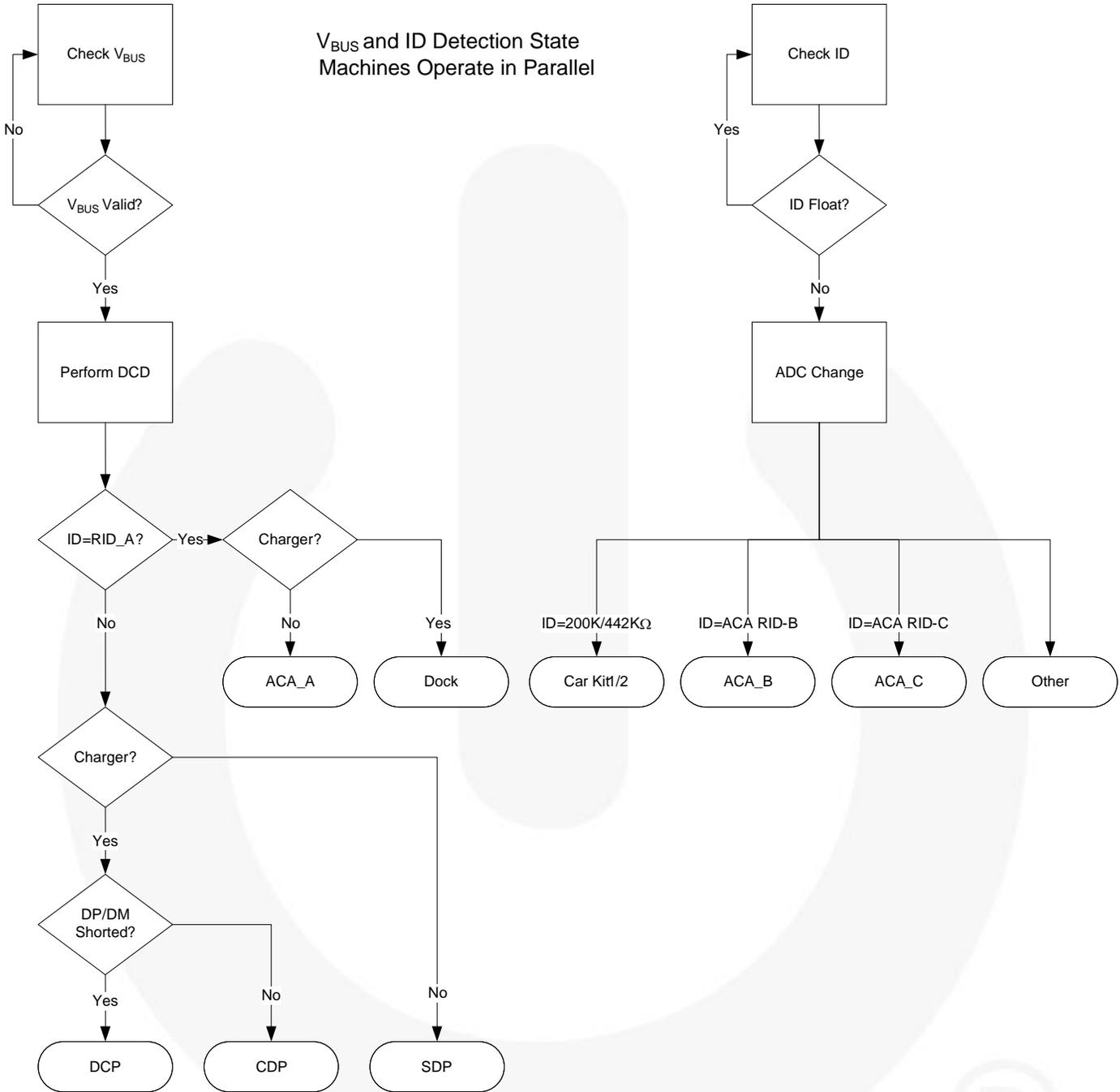
**Figure 5. Accessory Discovery State Machine Flow Diagram**
