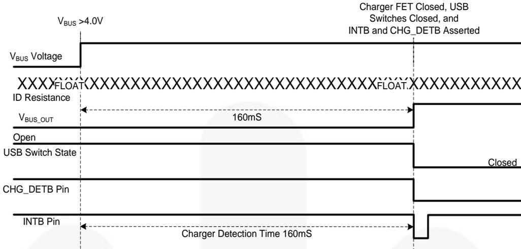
Figure 10. USB Dedicated Charging Port (DCP) or Charging Downstream Port (CDP) Attach Timing<sup>(20)</sup>
