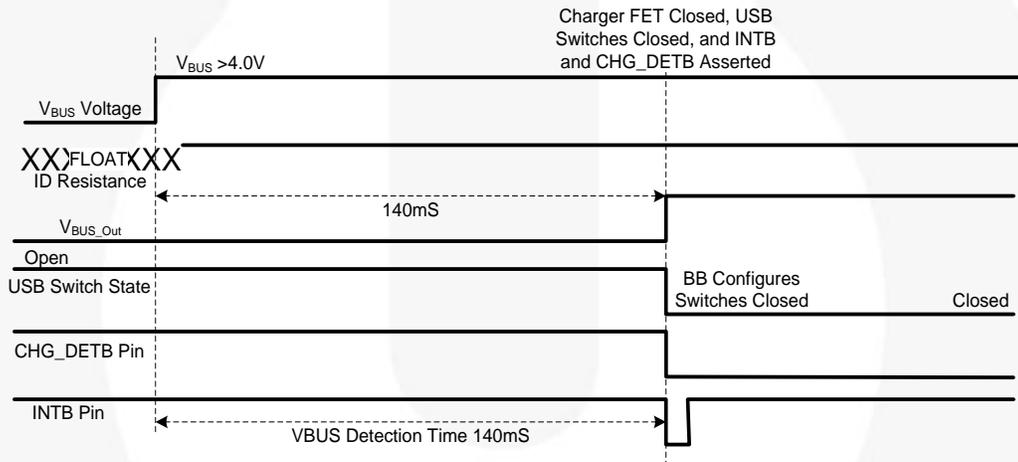
Figure 11. Car Kit Type-1 and Type-2 Attach Timing
