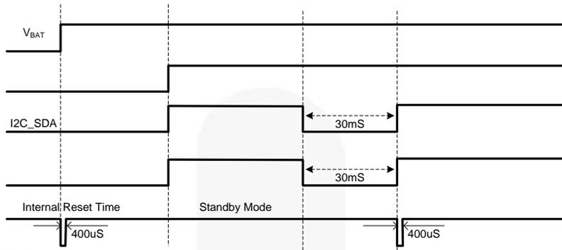
Figure 7. I<sup>2</sup>C Reset Mode Timing
