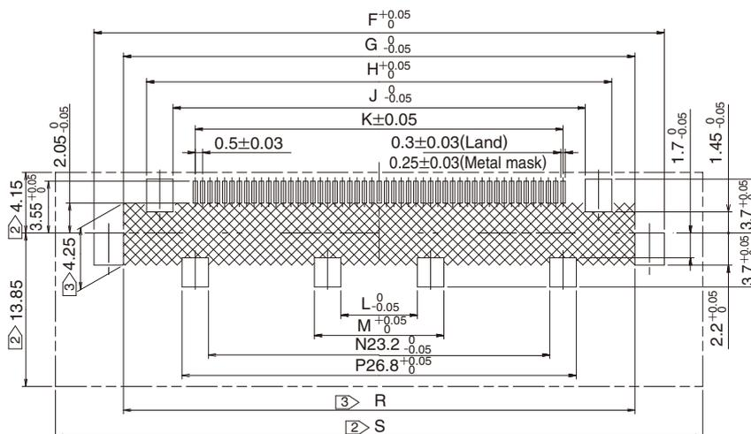
Note 1 : The coplanarity of the terminal leads is 0.1mm max. for all signal leads and 0.15mm max. for the shield leads.
