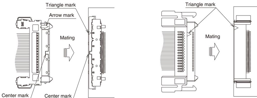
Additionally, this connector is equipped with reverse-insertion preventing mechanism, but a forced mating with a minimum force of 25N could damage the connector. Avoid any inappropriate mating, and perform the mating operation after checking the above-mentioned polarity indication.
