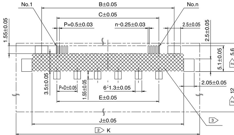
Note 1 : The coplanarity of the terminal leads is 0.1mm max.
