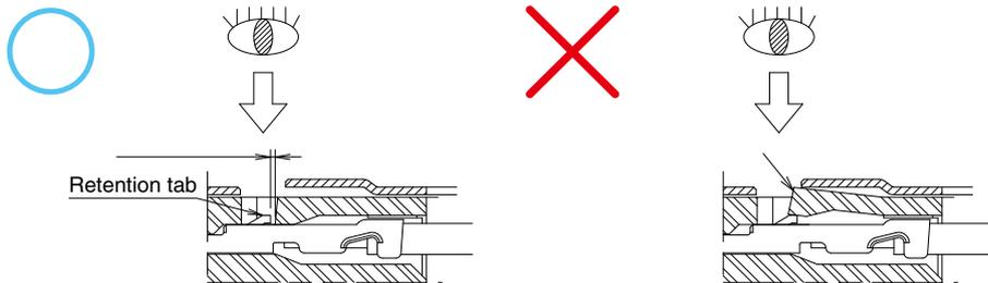
Light pull on the wire, with force NOT EXCEEDING 3N will also verify the correct contact insertion.
