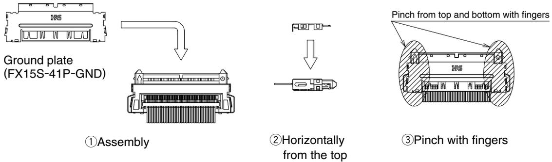
3. Check the six fitting points after assembly and make sure that they are all correctly fitted together.
