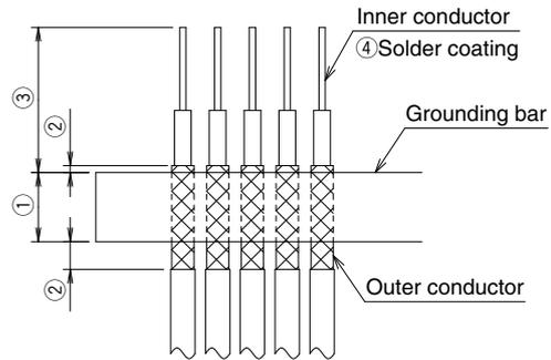
2. Recommended solder for the assembly is flux cored solder with 0.2mm dia. (Lead-free: Sn-3Ag-0.5Cu), 21mm length. If additional flux is used, make sure to prevent wicking onto the contact area. Wicking onto the contact area will cause the contacts to fail.
