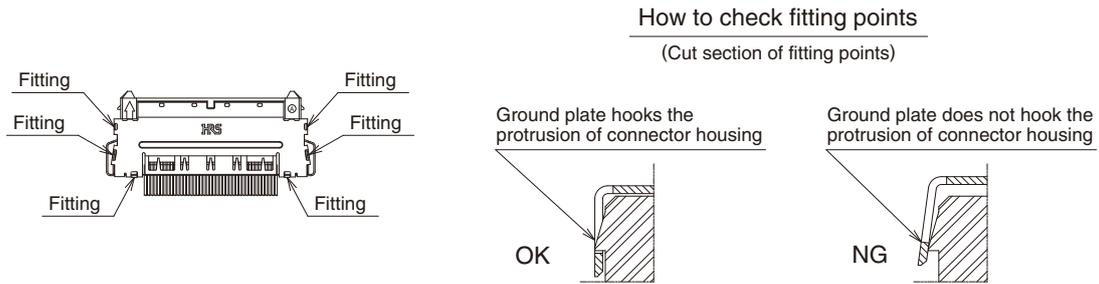
[ Soldering to ground plate ]
