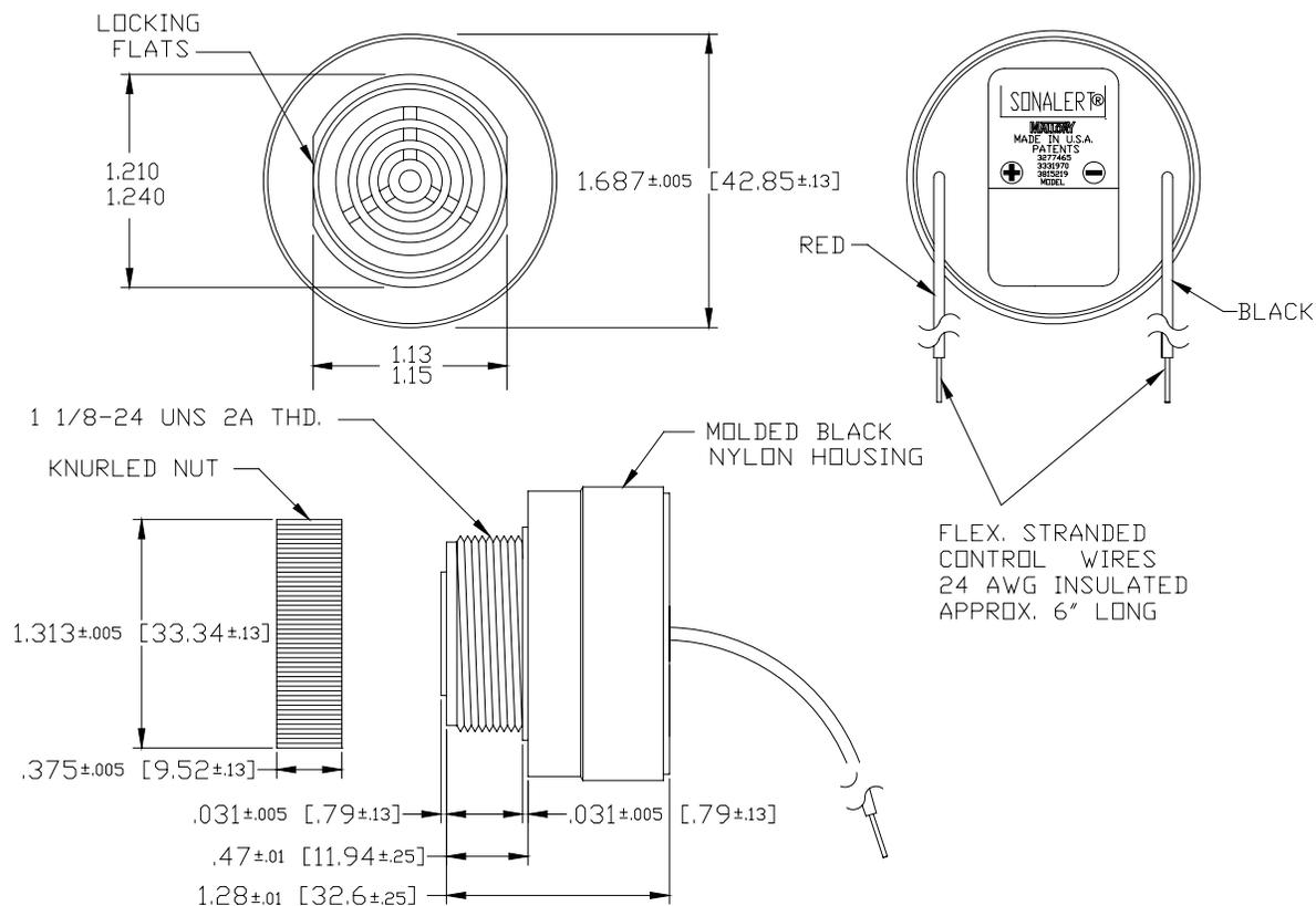
NOTE: MOUNTING- REMOVE BLACK PLASTIC NUT AND INSERT THREADED FRONT THROUGH 1.25" HOLE PUNCHED IN PANEL, IF ORIENTATION
