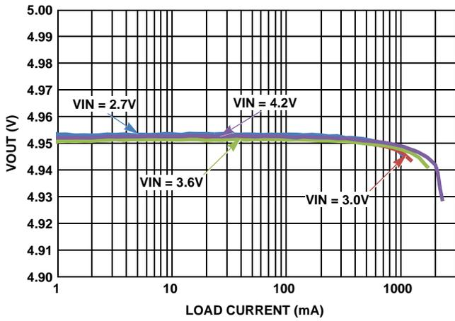
FIGURE 9. OUTPUT VOLTAGE vs LOAD CURRENT
