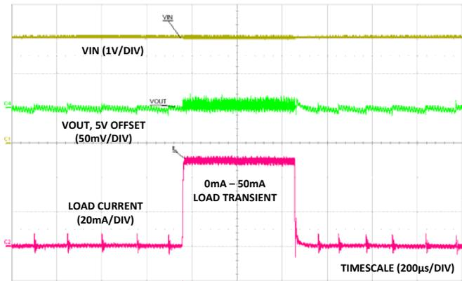
FIGURE 13. LOAD TRANSIENT ( $V_{IN} = 3.0\text{V}$ ,  $V_{OUT} = 5\text{V}$ )
