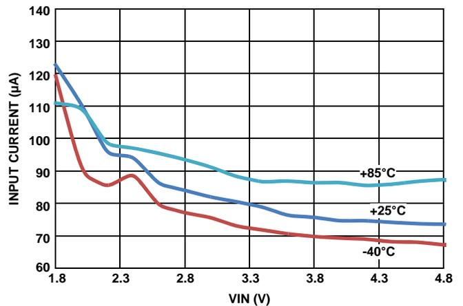
FIGURE 6. INPUT CURRENT vs INPUT VOLTAGE (MODE = HIGH)
