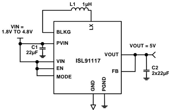
FIGURE 1. TYPICAL FIXED OUTPUT APPLICATION
