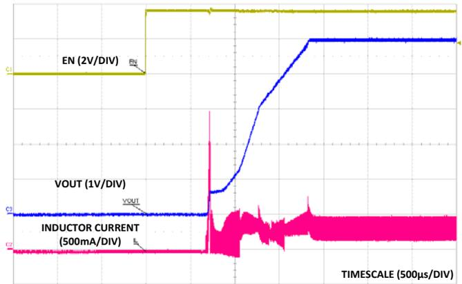
FIGURE 18. START-UP WITH 25Ω (VIN = 3.6V, VOUT = 5V)
