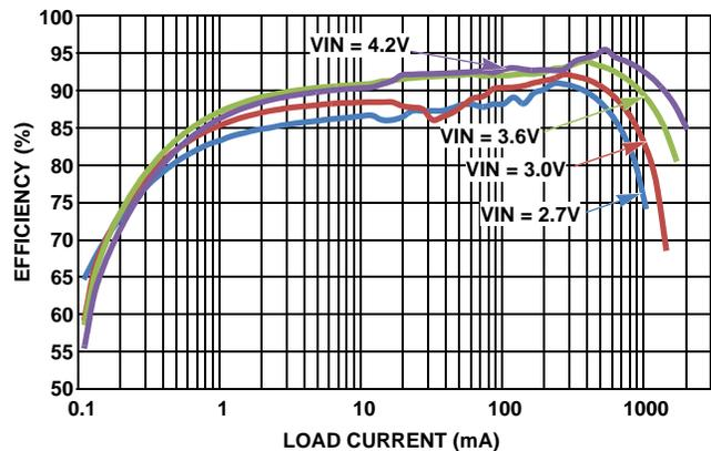
FIGURE 2. EFFICIENCY vs LOAD CURRENT ( $V_{OUT} = 5V$ )
