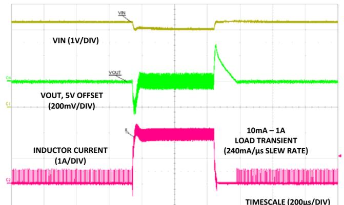
FIGURE 14. LOAD TRANSIENT ( $V_{IN} = 3.0\text{V}$ ,  $V_{OUT} = 5\text{V}$ )
