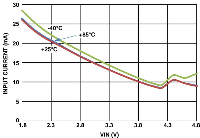
FIGURE 7. INPUT CURRENT vs INPUT VOLTAGE (MODE = LOW)
