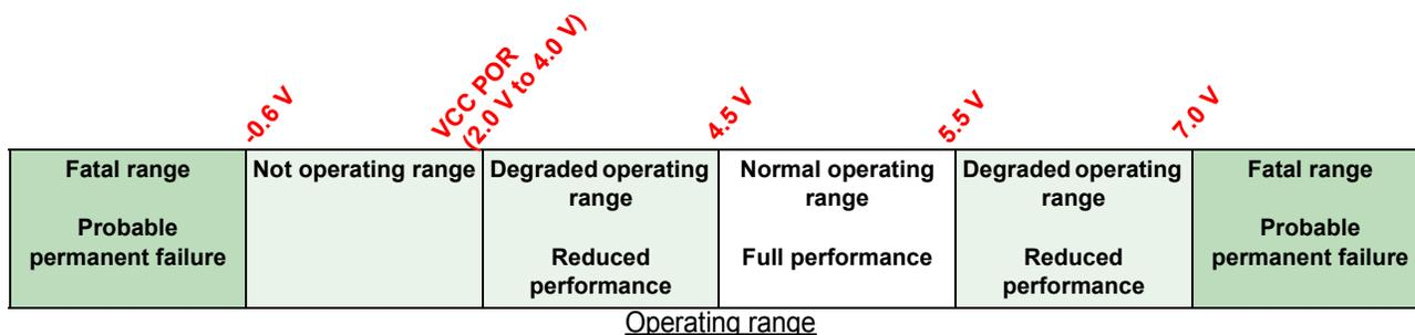
Figure 5. Ratings vs. operating requirements (VCC pin)
