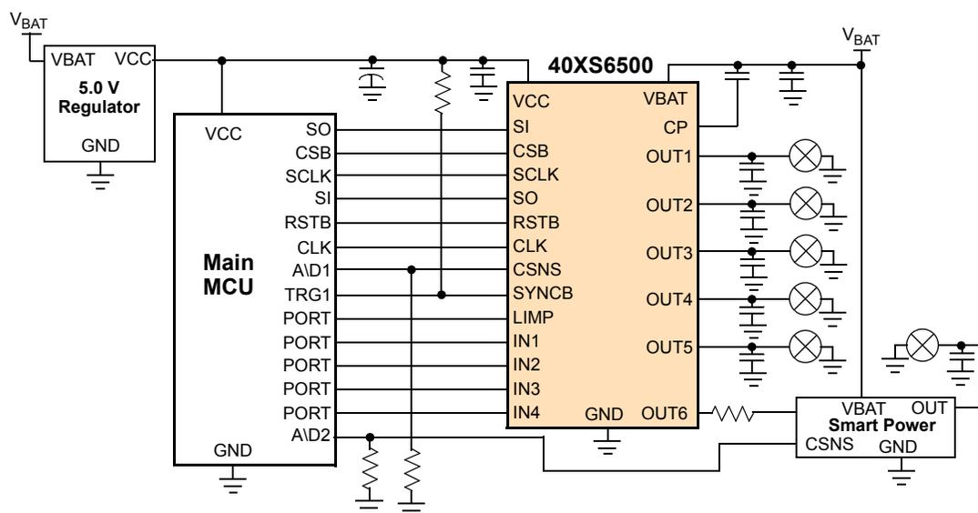
Figure 1. Penta 40 mΩ high-side simplified application diagram
