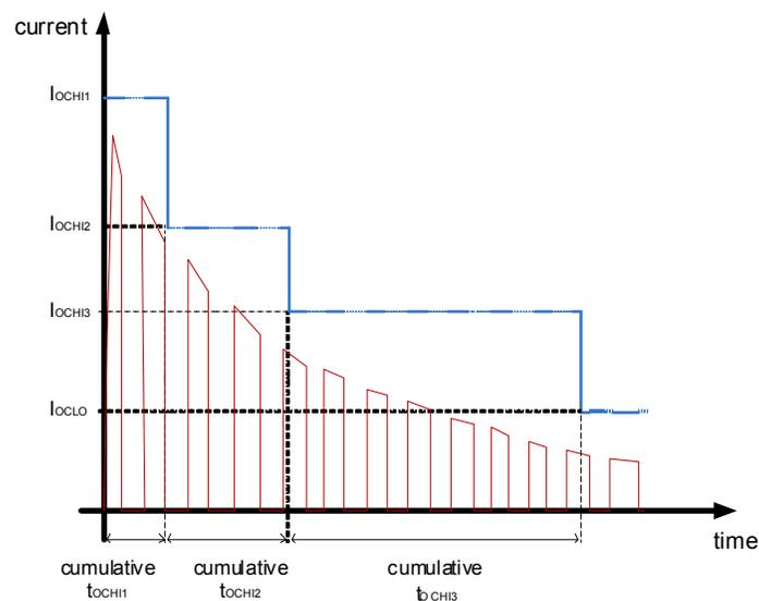
**Figure 15. Transient overcurrent profile in PWM mode**
