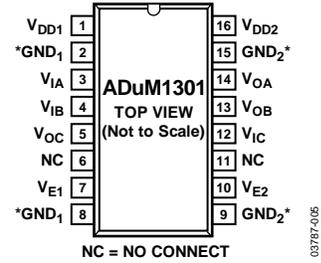
\*PIN 2 AND PIN 8 ARE INTERNALLY CONNECTED, AND CONNECTING BOTH TO GND<sub>1</sub> IS RECOMMENDED. PIN 9 AND PIN 15 ARE INTERNALLY CONNECTED, AND CONNECTING BOTH TO GND<sub>2</sub> IS RECOMMENDED.
