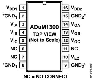
\*PIN 2 AND PIN 8 ARE INTERNALLY CONNECTED, AND CONNECTING BOTH TO GND<sub>1</sub> IS RECOMMENDED. PIN 9 AND PIN 15 ARE INTERNALLY CONNECTED, AND CONNECTING BOTH TO GND<sub>2</sub> IS RECOMMENDED.
