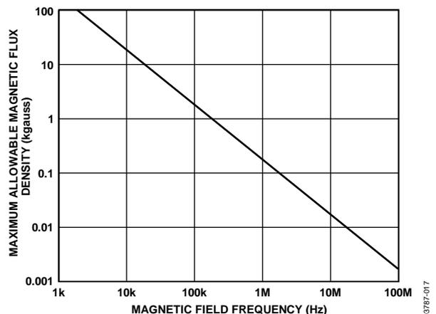
Figure 16. Maximum Allowable External Magnetic Flux Density
