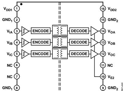
Figure 1. ADuM1300 Functional Block Diagram
