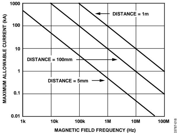
Figure 17. Maximum Allowable Current for Various Current-to-ADuM1300/ADuM1301 Spacings
