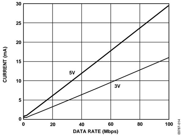
Figure 12. Typical ADuM1301 V<sub>DD2</sub> Supply Current vs. Data Rate for 5V and 3V Operation
