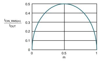
Figure 1. I<sub>CIN</sub> vs. Voltage Conversion Ratio
