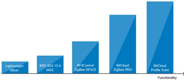
The Lightweight Mesh software stack is designed to work with all Atmel IEEE 802.15.4 transceivers and SoCs. Currently the stack works with Atmel AVR<sup>®</sup> microcontrollers (MCUs), but given its extreme portability and low resource requirements, it can be run on almost any Atmel MCU. For more details, visit [www.atmel.com/tools/LIGHTWEIGHT\\_MESH.aspx](http://www.atmel.com/tools/LIGHTWEIGHT_MESH.aspx).
